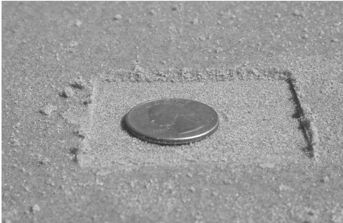
Figure 3.4 Sample taken to field calibrate the spectroradiometer. Coin shown for scale is 24 mm in diameter and approximately 1.5 mm thick.
