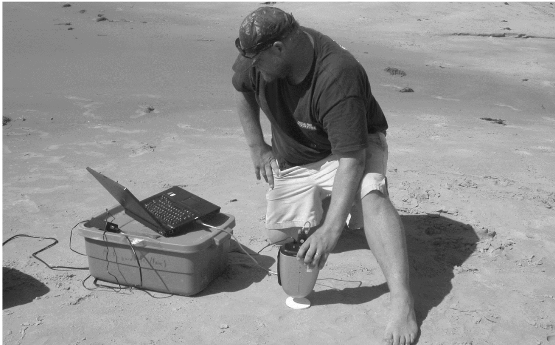
Figure 3.2 Spectroradiometer being used to collect a white reference measurement at North Padre Island, TX. Note the shadow over the panel. This is unavoidable in the field, but as long as measurement geometry is not significantly altered between white reference and actual sample measurements (about 10 seconds apart), this is not a major issue.
