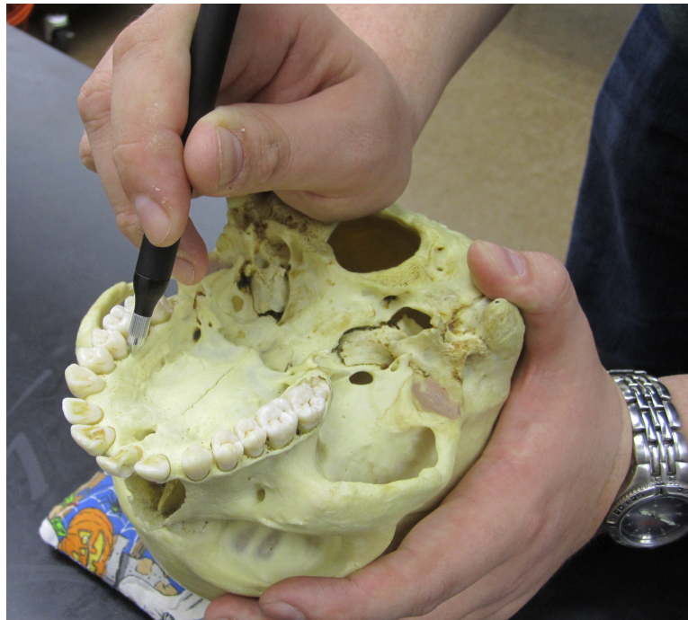
Figure 1: Photograph of how the points are recorded using the digitizer.
