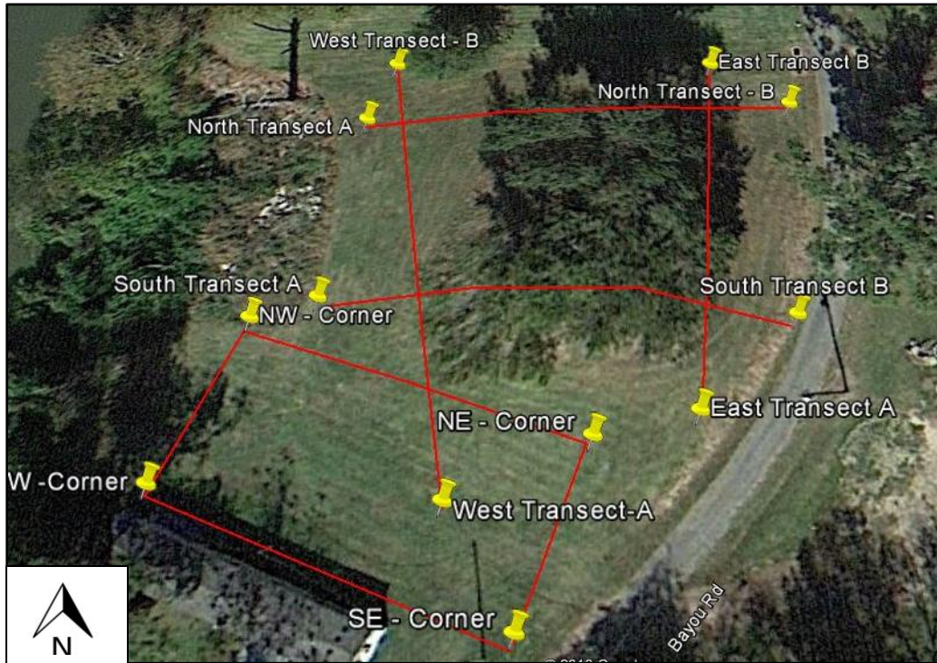
Figure 4-1. Google Aerial View of Area A and Pseudosection Lines Drawn across the mound.
