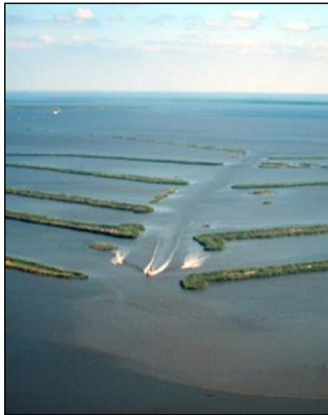
Figure 2.5: Terraces encourage sediment deposition and protect existing wetlands by reducing wave action in the shallow waters of Little Vermillion Bay, Louisiana (NOAA 2004)
