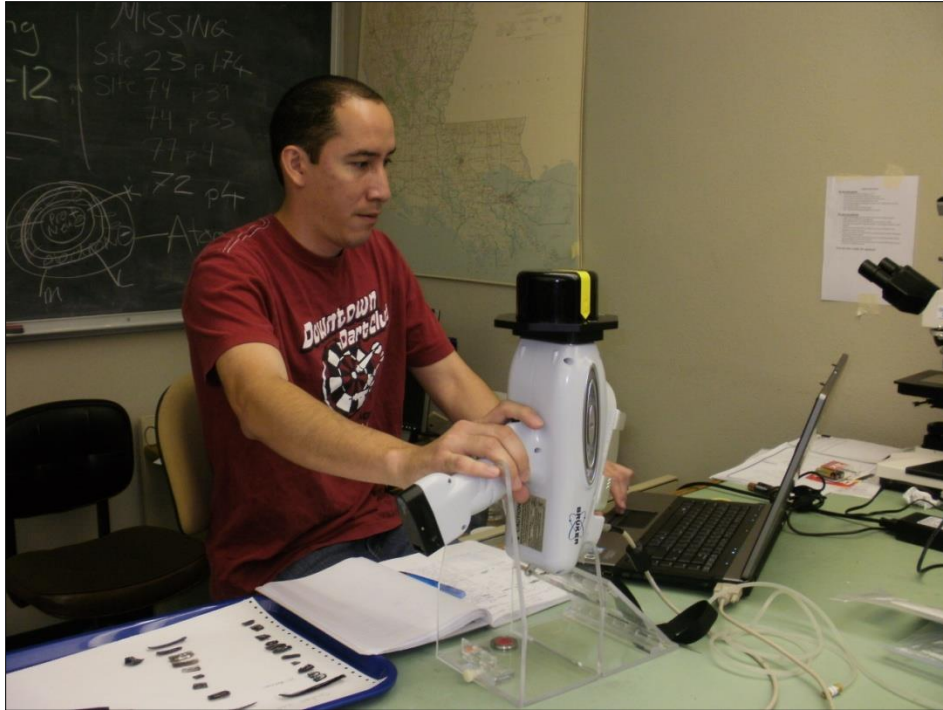
Figure 29. Roberto Rosado arraying an obsidian blade in the Coastal Archaeology Lab with the Bruker Tracer 3-V (photo by H. McKillop).
