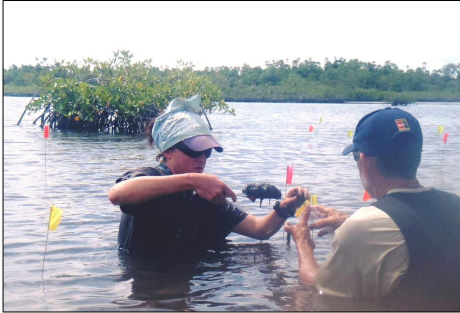
Figure 21. Photograph of acquiring the marine sediment samples at Chan B'i using a stainless steel knife and placing the sediment into Whirl-pak bags (photo by H. McKillop).
