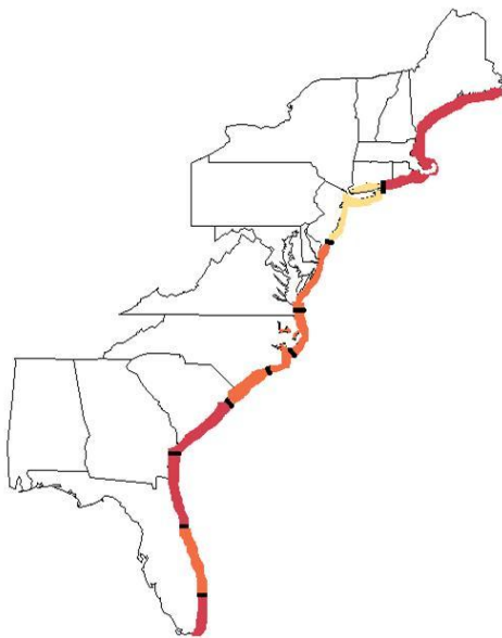
Figure 4.5: Comparison of regions based on 100-year quantile estimate. Red zones have a 100-year event > 4.6 m (15 ft); orange zones have a 100-year event > 3.05 m (10 ft) but < 4.6 m; yellow zones have a 100-year event < 3.05 m.
