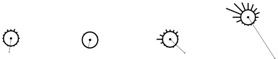
Figure 2.16. Spring, summer, fall, and winter sand roses (from left to right) for sample location 9 as indicated on Figure 2.2. Sample 9 had the highest mean grain size and threshold velocity of the twelve samples taken at the Jinx blowout.
