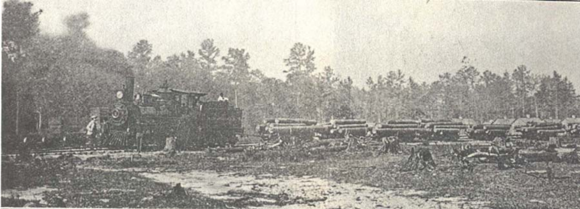
FIGURE 4.5. THE GREENLAW LUMBER COMPANY, 1905; THIS PHOTO SHOWS HOW LUMBER WORKERS USED THE RAIL LINES TO HAUL CUT LOGS. THE LOGS WOULD HAVE BEEN TAKEN TO A SAW MILL, CUT INTO LUMBER, AND THEN SHIPPED BY RAIL OR BARGE TO MARKETS OUT OF STATE. THE FOREGROUND GIVES AN INDICATION OF HOW THE DENUED LANDSCAPE APPEARED. FROM THE WORLD FAMOUS OZONE BELT , 1905.
