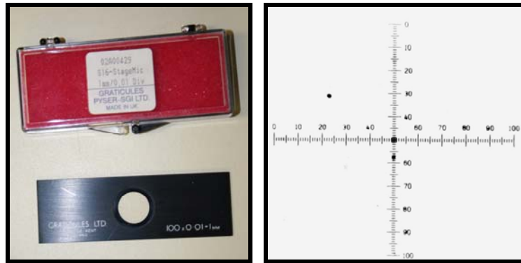
Figure 3.10a (left): Graticules Pyser-SGI Ltd ® Calibrating Slide 1mm/0.01 Divisions. Figure 3.10b (right): 1mm/0.01 Calibration Image.
