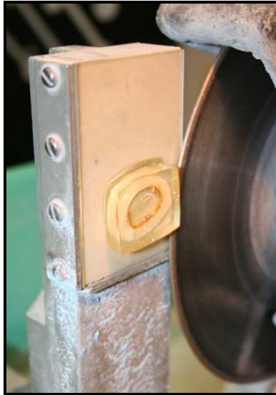
Figure 3.7: Slicing of 1mm Sample from the Histoblock on the Resectioning Saw.
