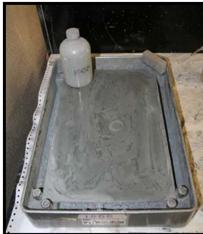
Figure 3.8: Glass pane with Polishing 1000 grit Silicon Carbide Powder.
