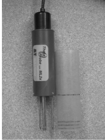
Figure 3.4: Cylindrical tube utilized to collect field moisture measurement samples. Rings on the tube indicate depth of measurement collection.
