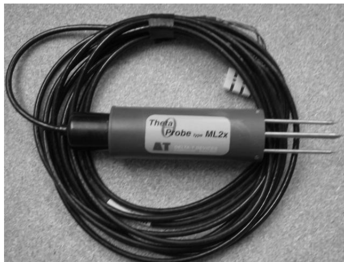
Figure 1.1: Delta-T Theta Probe soil moisture sensor Photo by: Phillip Schmutz
