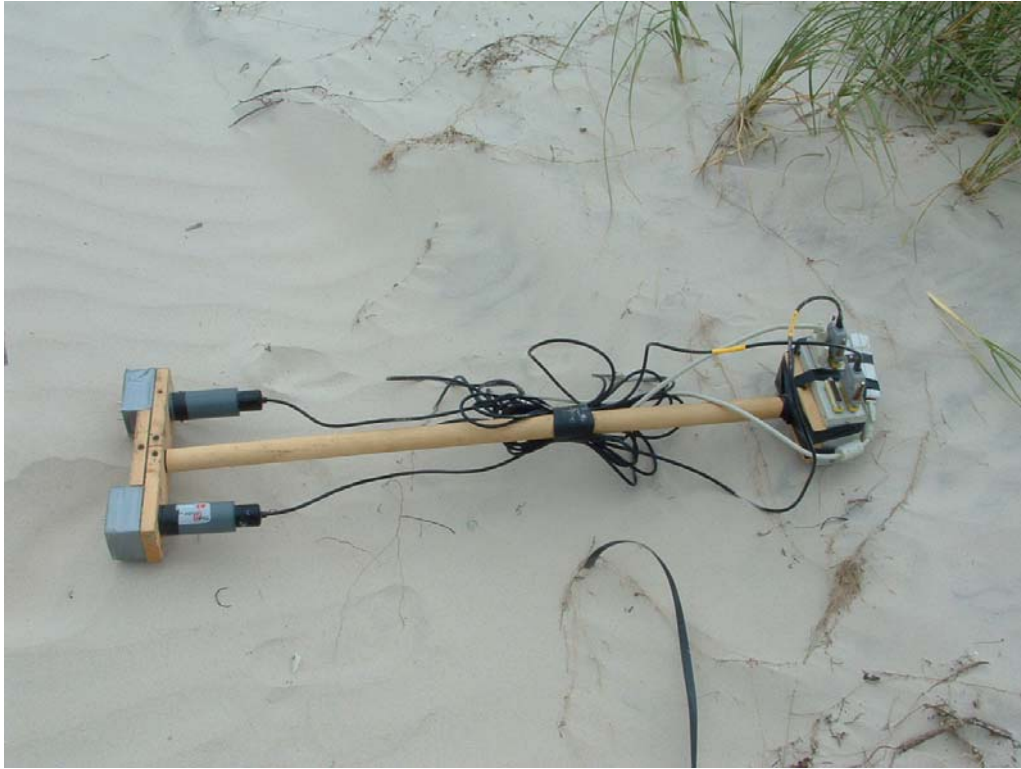
Figure 3.6 Photo of moisture probes and the wooden platform used to measure surface moisture content
