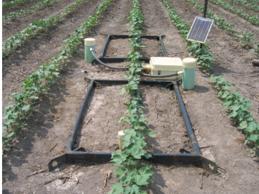
Figure 3.2 Weighing lysimeters with developing cotton crop (Clawson et al. , 2009)
