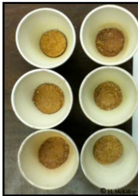
Figure 10. Inorganic content left after the loss-on ignition procedure.
