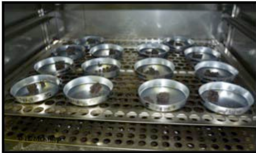
Figure 6. Samples from Site 35 drying in the oven.
