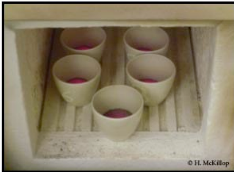
Figure 8. Samples at 500° Celsius in the furnace. Photo by J. Harrison.
