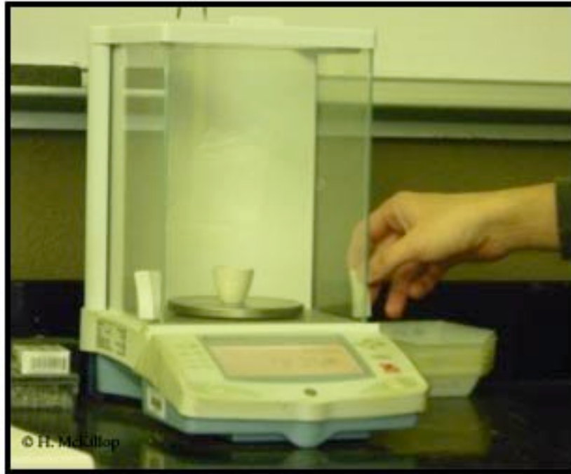
Figure 9. Weighing samples after the loss-on ignition procedure.
