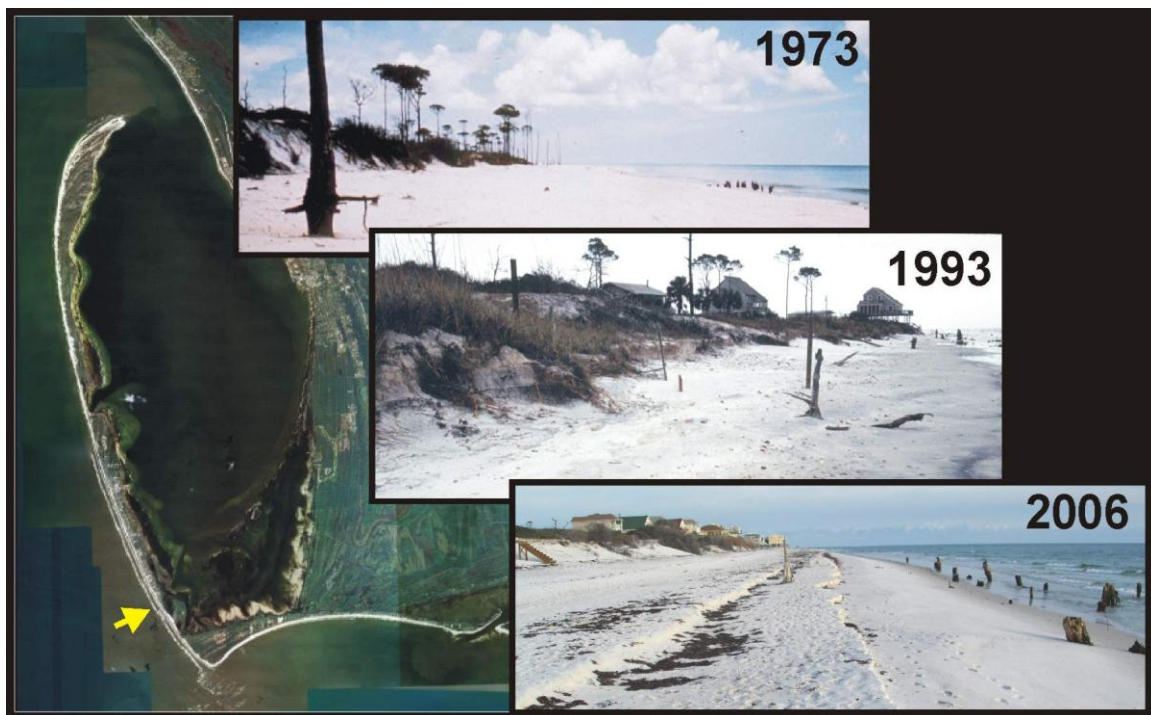
Figure 5.26 – Profile R100. Beach erosion as indicated by seaward tree stumps, has been accompanied by retreat and loss of the foredune.
