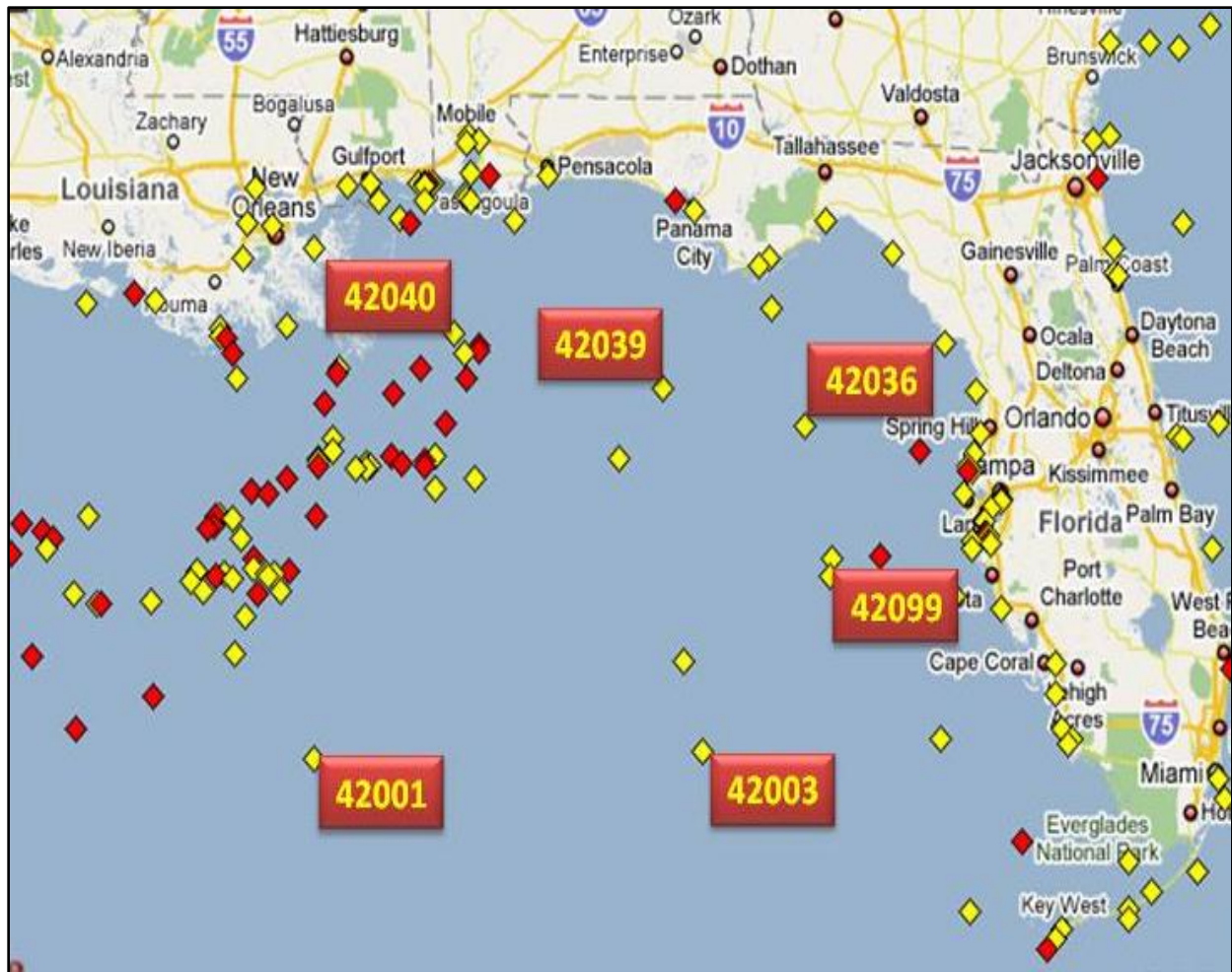
Figure 4.5 –NDBC Buoy locations for comparing actual wave parameters with MIKE-21 calculated wave parameters. Image source: Modified from NOAA NDBC website (2010).
