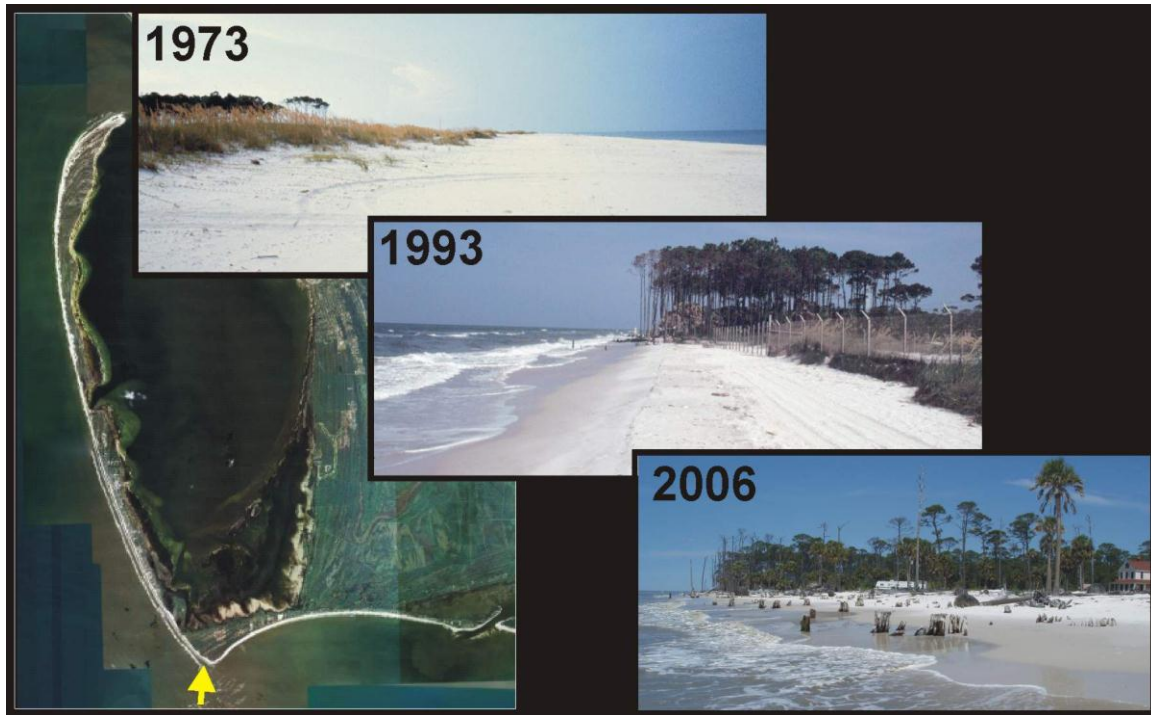
Figure 5.28 – Profile R110. The 1973 view (looking east) displays the wide beach and foredune present on the 1973 profile. Following extensive erosion, the 1993 (looking west from R112) and the 2006 (looking west) photo show no foredune and continued beach erosion.
