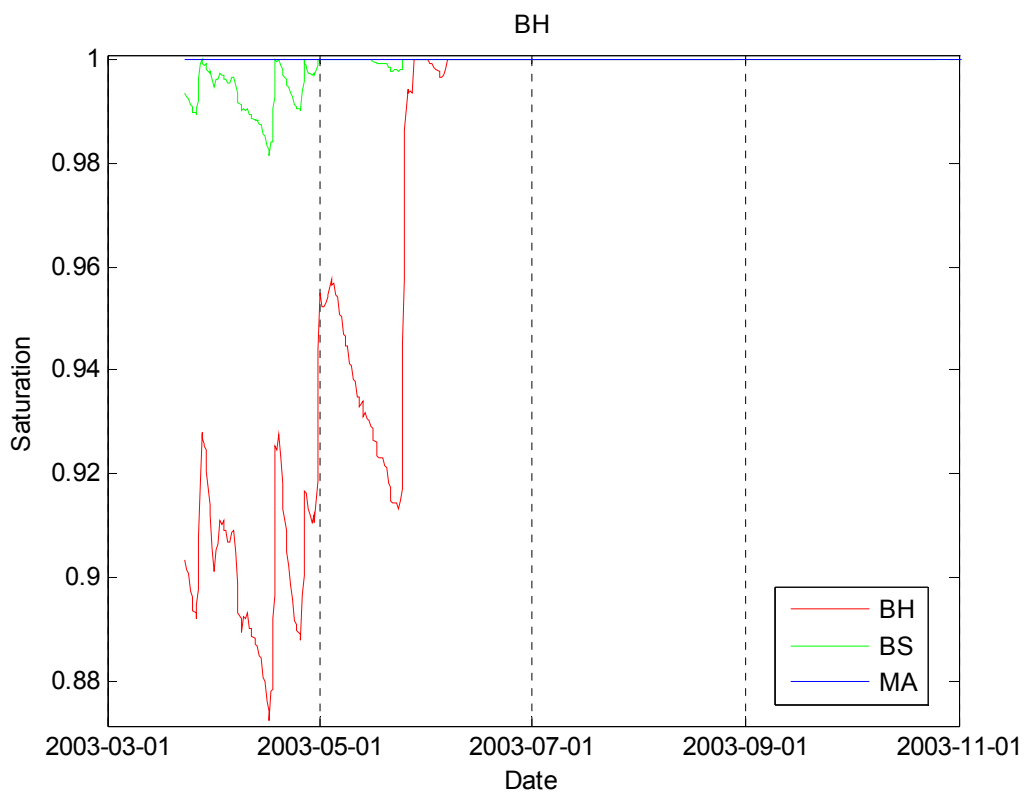
Figure A-73. Water table level and soil saturation obtained from the model for Black Hammock wells for the case K1. It is comparable to Figure A-64 for case K0.
