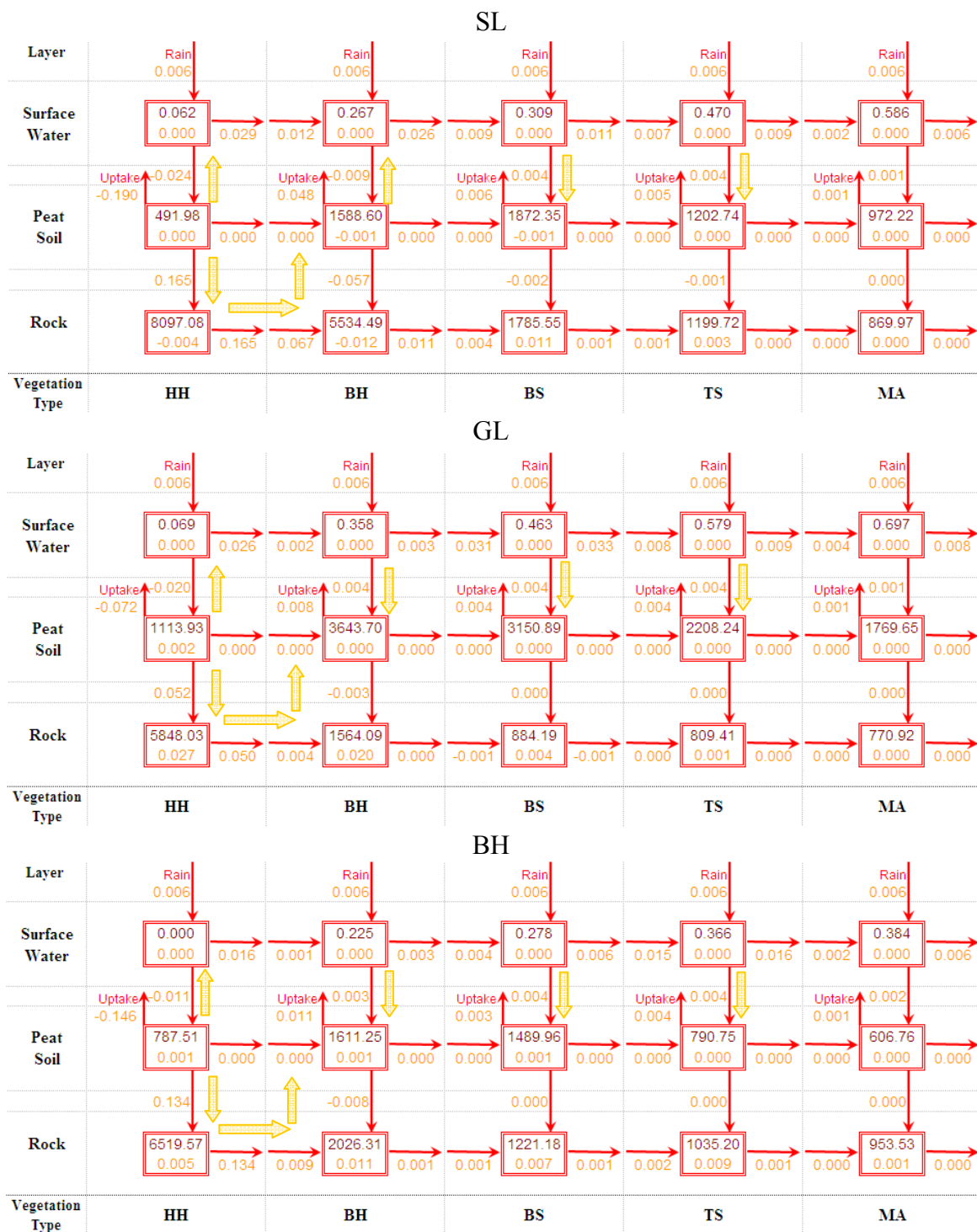
Figure 71. Pools and fluxes of dissolved and adsorbed Phosphorus mass in the model after a 10 year simulation for each tree island for case L0. Pools amounts are in mgP/m 2 and fluxes in mgP/m 2 /day units.
