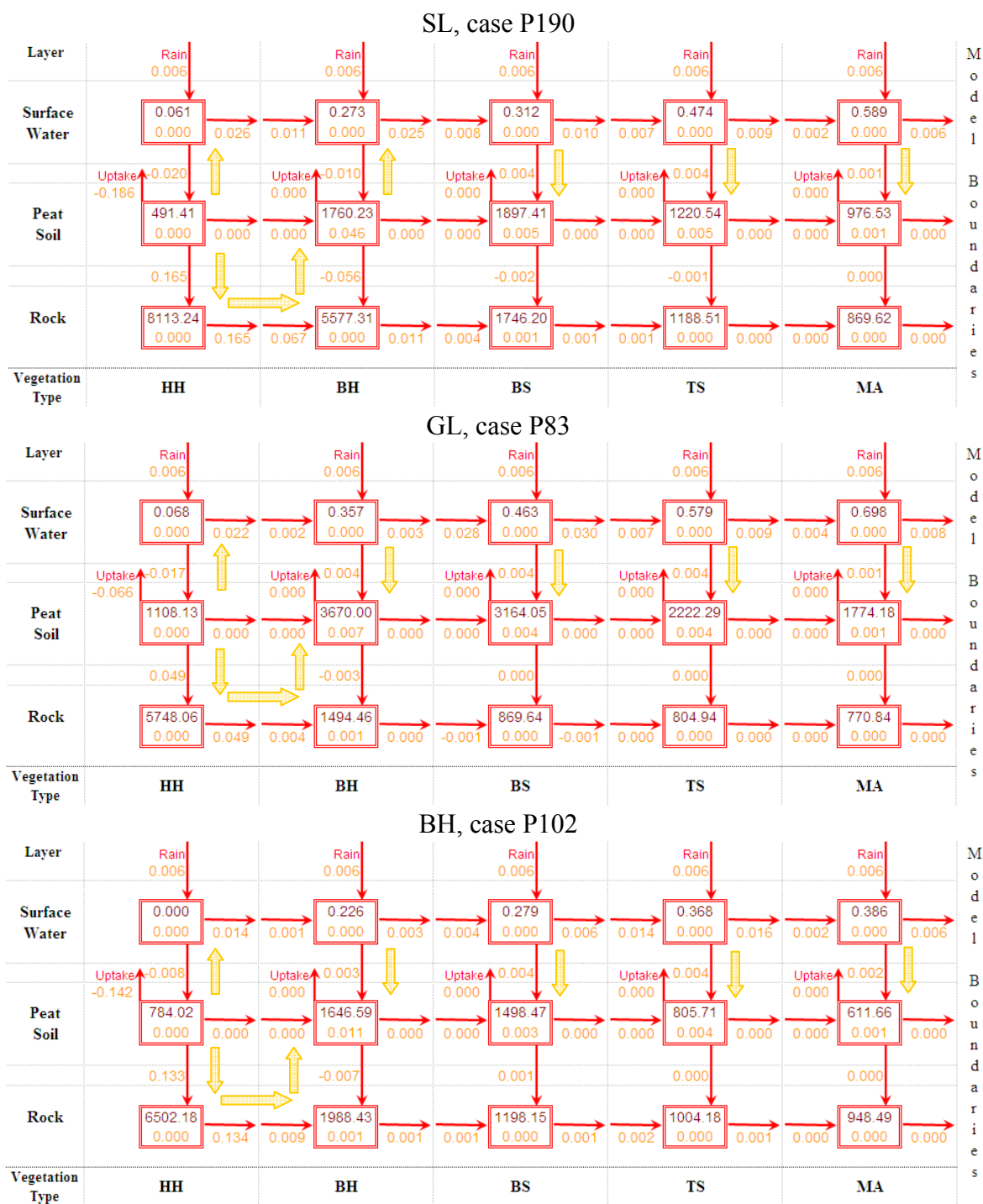
Figure 68. Pools and fluxes of dissolved and adsorbed Phosphorus mass in the model after a 10 year simulation for each tree island. Pool mass values for each layer and vegetation type are presented in dark red correspond to the end of the simulation. They are normalized by unit horizontal area ( \text{mg}/\text{m}^2 ). Mass flux values presented in pink correspond to the average over the 10 years, and they are also normalized by unit horizontal area ( \text{mg}/\text{m}^2/\text{day} ).
