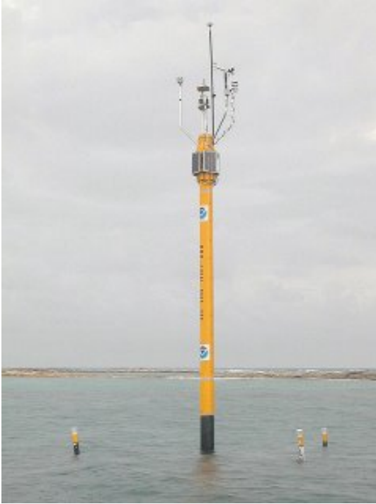
Figure 3.4 A picture of station pylon at LPPR1 stations, the light and atmospheric instruments are located on top at about 6.5 m height.
