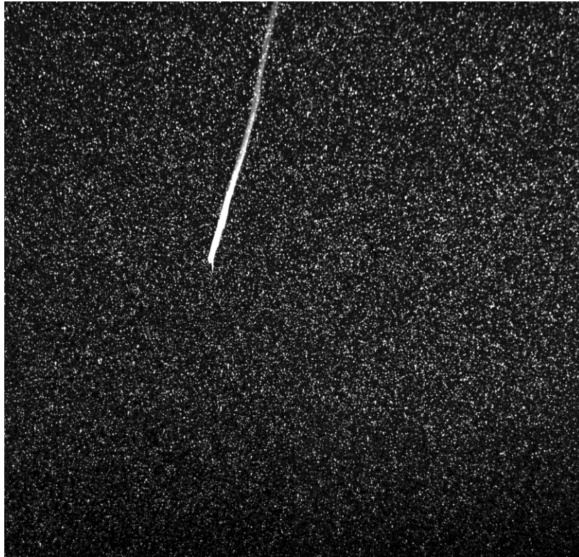
Figure 2.9. Sample PIV image (20 cm high by 26 cm across) showing the flow seeded with 10 \mu\text{m} particles. The white streak extending from the top into the center of the tank is a thermistor in the cell interior. The apparent vertical gradient in particles is an artifact due to weaker laser intensity near the bottom of the tank. Pairs of such images are cross-correlated to track movement of the particles, and so obtain velocity flow fields for the tank cross section.
