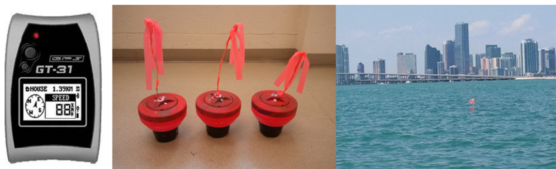
Figure 13: Left: Loicosys GT-31 portable GPS; Middle: Drifter; Right: Drifters in Biscayne Bay off of Hobie Beach.
