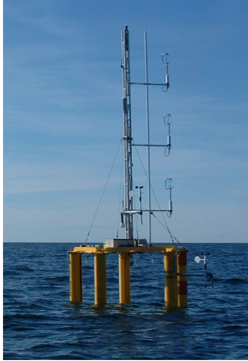
Figure 3.1: The fully-loaded ASIS buoy as deployed during a field experiment. Three Sonic anemometers and two thermistors are installed on ASIS buoy.
