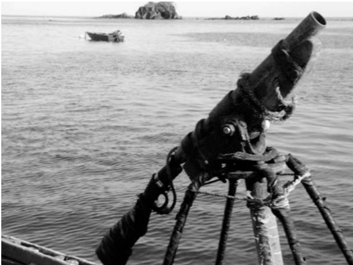
Figure 5.22: Shotgun modified for firing harpoons, mounted on the bow of the Sea Hunter .
