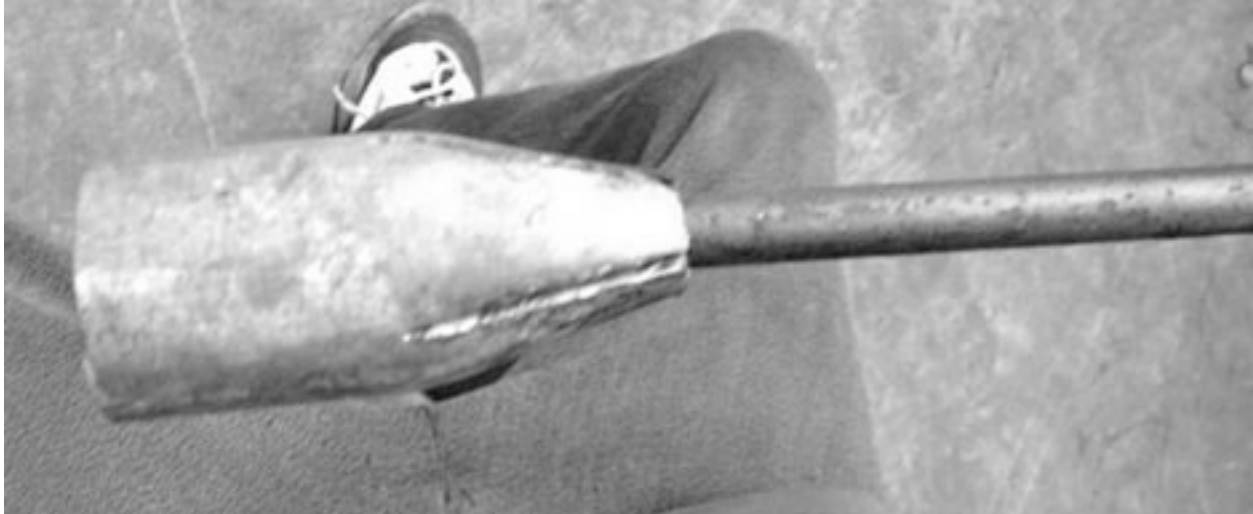
Figure 5.17: A harpoon foreshaft welded to the cup that will attach to the main shaft.
