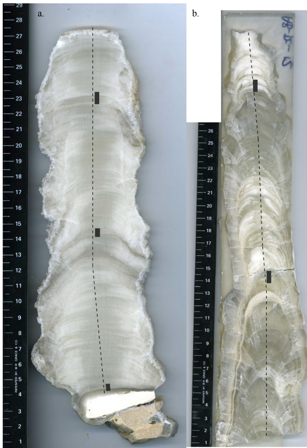
Figure 6.3: Reflected light photos of samples AB-DC-09 (a) and AB-DC-12 (b). For both a and b: Dotted line is the location of low resolution (1000 \mu\text{m} ) sampling and black squares are the sampling locations for the high resolution (20 \mu\text{m} ) analysis.
