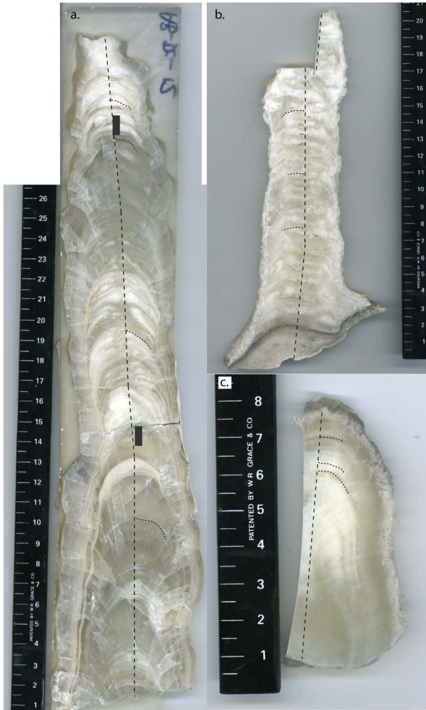
Figure 4.3: Photos of samples utilized in this study. A) Sample AB-DC-12, B) Sample AB-DC-03 and C) Sample AB-DC-01. All samples were analyzed at a low resolution (dotted vertical line) and Hendy tests were conducted (horizontal dotted line). Sample AB-DC-12 was analyzed at high resolution at two locations (black squares).
