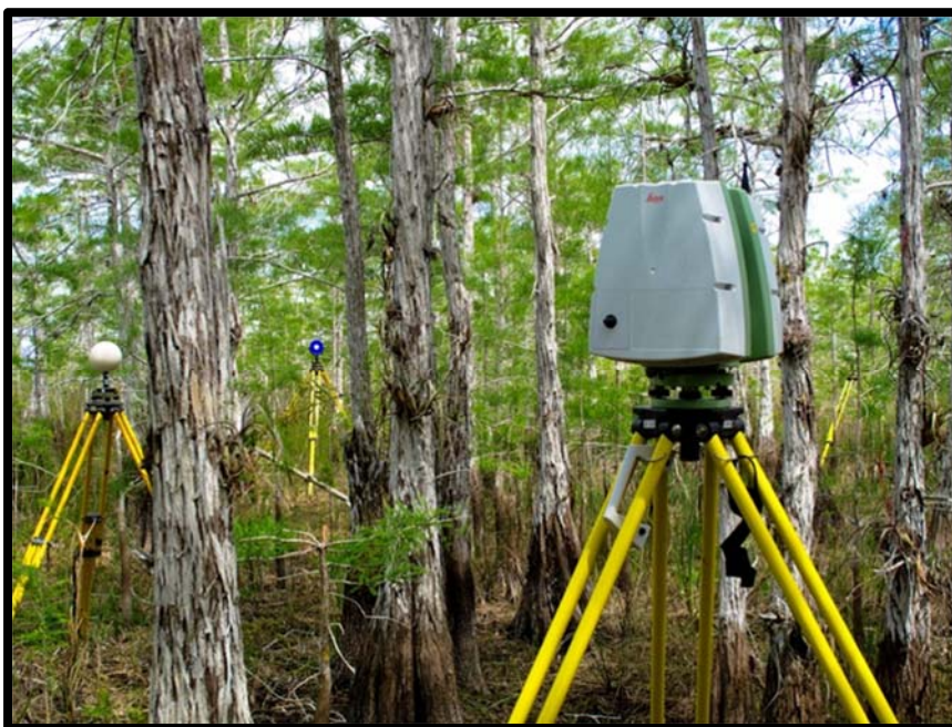
Figure 5.2 Leica ScanStation C10 TLS in ENP bald cypress site. Three targets can be seen scattered in the cypress forest.
