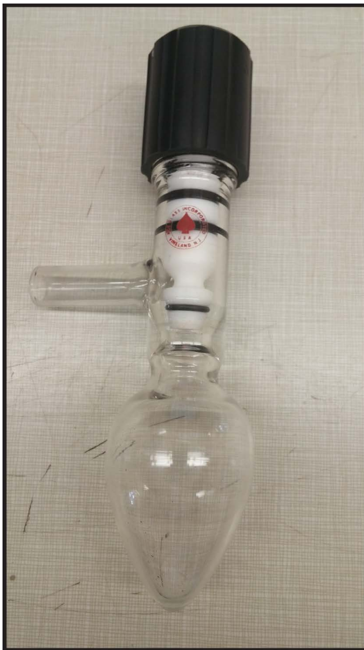
Figure 1.6 – Pear-shaped vessel used in both the transferring of sample CO 2 gas from the vacuum line to the mass spectrometer and in all the sealed vessel reactions.
