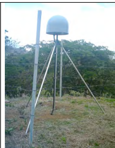
Figure A.9 HATI is built to the specifications of PBO. It is a short-drilled monument where each bracing leg reaches depths of ~1.5 m to maximize coupling. GRZA is equipped with a Trimble Choke Ring antenna with ray dome and a Trimble NetRS receiver.
