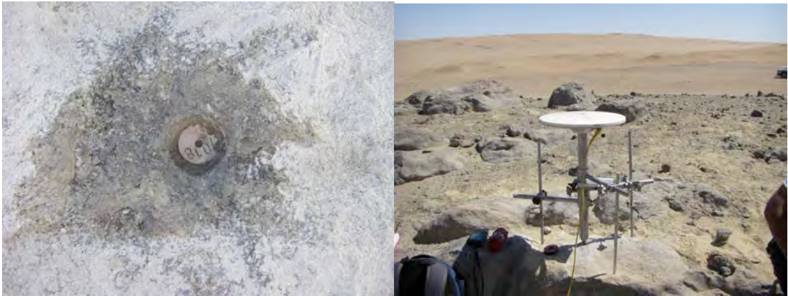
Figure 2.2. Representative pictures from a GPS campaign showing the monument pin and a spike mount set up with a Zephyr Geodetic antenna with ground plane.
