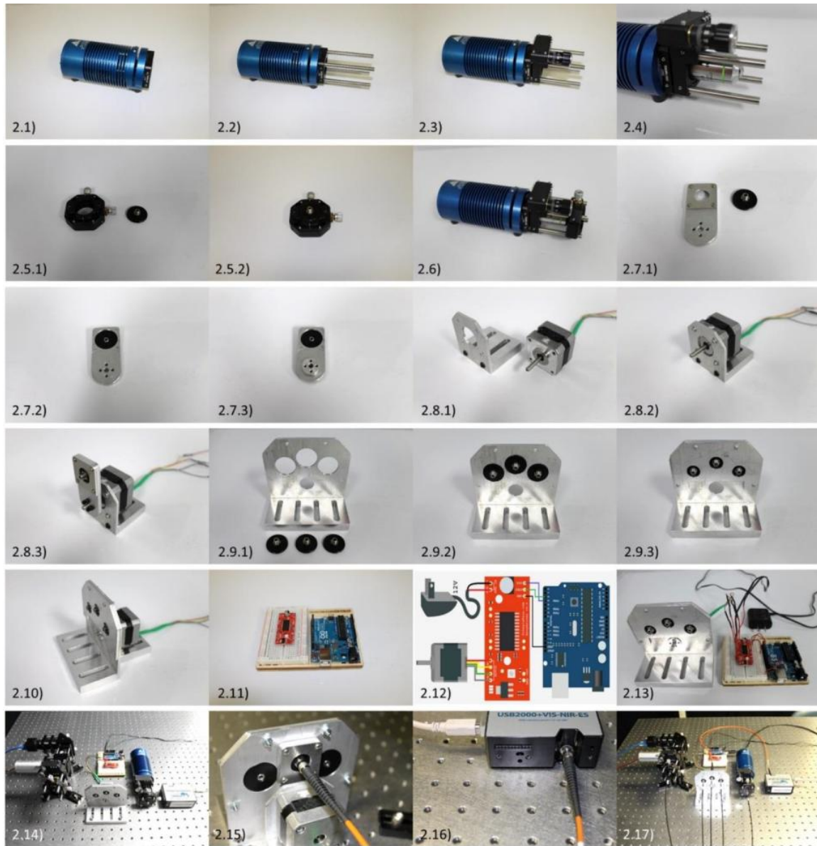
Figure 5. Assembly of the sub-diffuse reflectance spectroscopy modality. The sub-diffuse reflectance spectroscopy modality can be constructed using a basic tungsten-halogen lamp coupled to an objective lens to focus light through the 200 \mu\text{m} multimode delivery fiber, and a spectrometer. Additionally, a custom-built motorized optical switch can be constructed within the lamp-fiber-spectrometer path to switch between each SDS. Investigators using multiple spectrometers to acquire from multiple SDSs can bypass the optical switch component.
