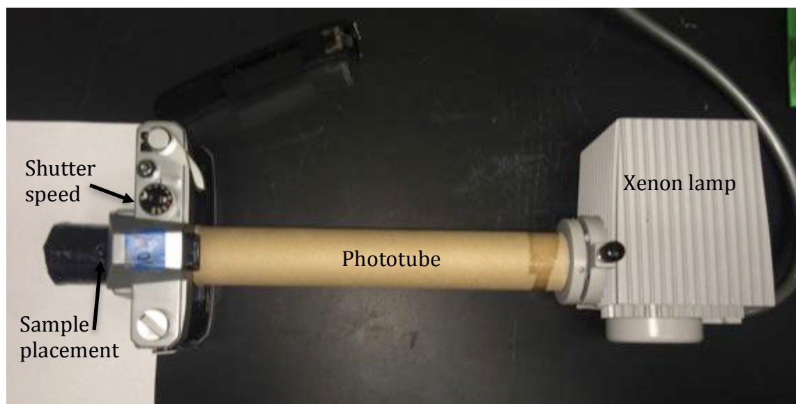
Figure 16: The photo-system used for performing PICUP on A\beta_{1-42} . The eppendorf tube containing the sample is placed in a small hole right in front of the camera. The amount of light exposed to the sample is controlled by the shutter speed. The phototube keeps the sample 9.875 inches from the Xenon lamp. This is estimated to be about 75 Joules of light.
