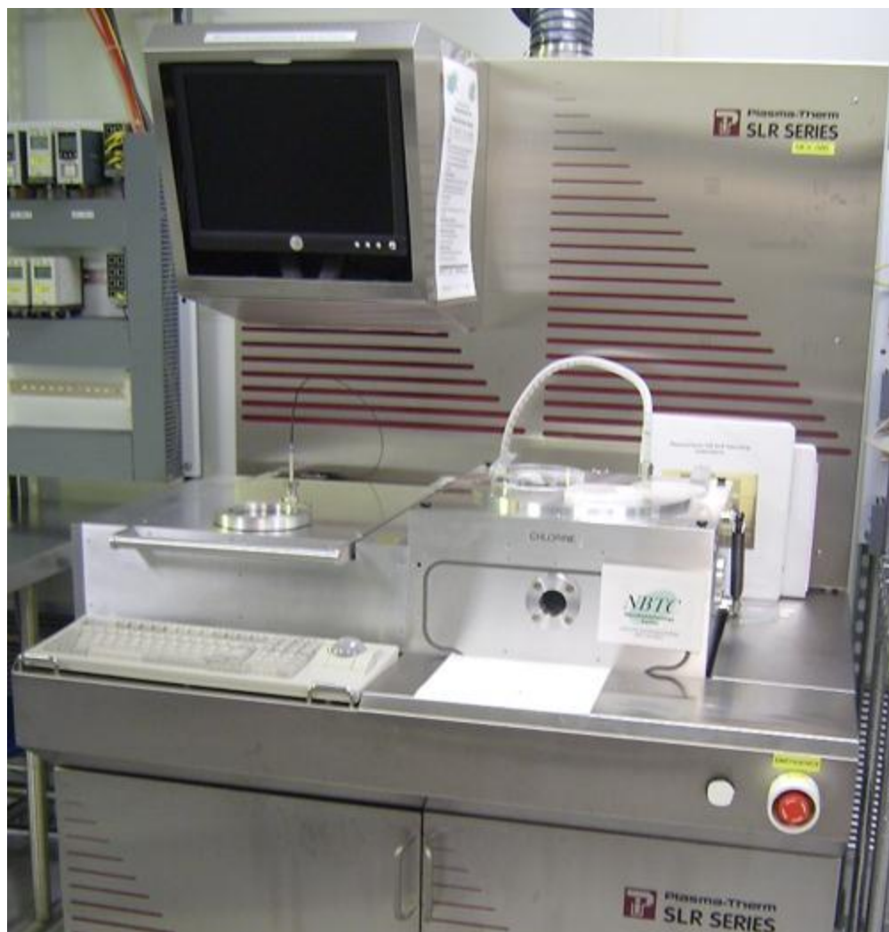
Fig. 4.9. Plasma treatment was conducted in the Plasma Therm SLR 720 RIE. Reactive Ion Etching with oxygen was performed at the University of Arkansas HIDEc center to introduce hydrophilic properties to the PCL scaffolds.
