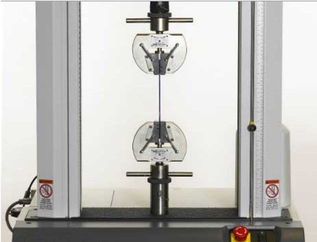
Fig. 5.1a. Instron 3365 system for determination of elasticity of electrospun scaffolds. Instron setup with clamps in order to test tensile strength and obtain a load curve for the test sample.
