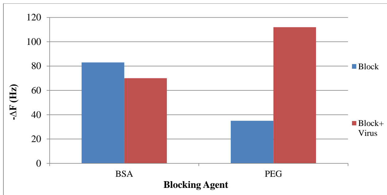
Figure 5.1- Frequency shifts of the QCM aptasensor comparing BSA and PEG blocking agents for AIV H5N1.
