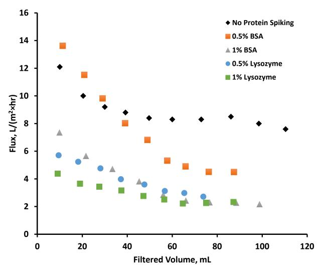
Figure 4. Flux measurement during Phi-X174 filtration using PES 100 kDa membrane in the absence and presence of lysozyme and BSA proteins at different concentrations.
