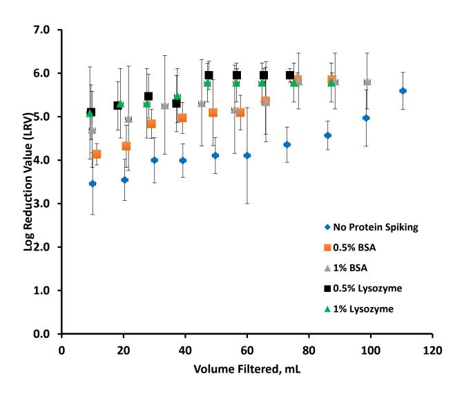
Figure 5. Titer analysis on each fraction collected from Phi-X174 filtration using PES 100 kDa membrane in the absence and presence of lysozyme and BSA proteins at different concentrations.
