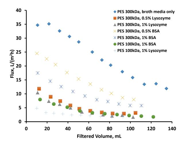
Figure 3. Flux measurement under different protein spiking conditions with PES 100 and 300 kDa membranes.
