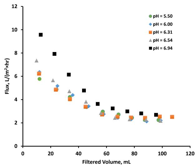
Figure 8. Flux measurement during Phi-X174 filtration using PES 100 kDa membrane spiked with 1% w/v BSA under multiple solution pH conditions.
