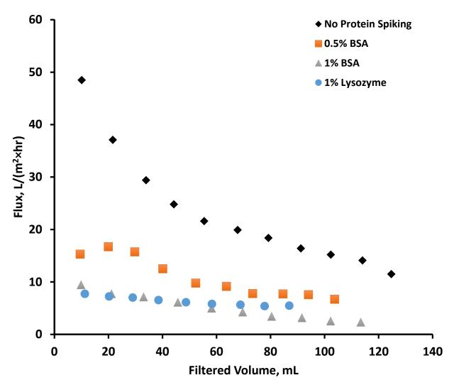
Figure 6. Flux measurement during Phi-X174 virus filtration using PES 300 kDa membrane in the absence and presence of lysozyme and BSA proteins at different concentrations.
