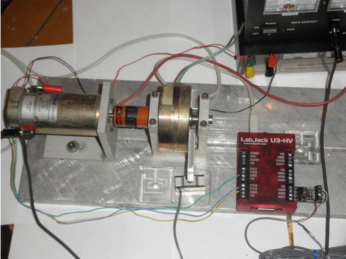
Figure 6.2. Dynamometer Setup with LabJack
