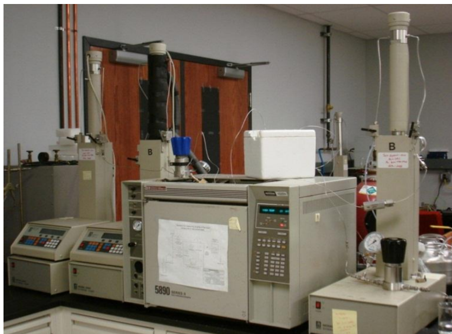
Figure 3.2: Photograph of lab-scale semi-continuous flow process unit
