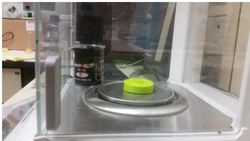
Figure 15. EP set-up with the scale, membrane sample cell, and activated carbon.
