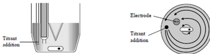
Figure 1. Appropriate mixing for titration
