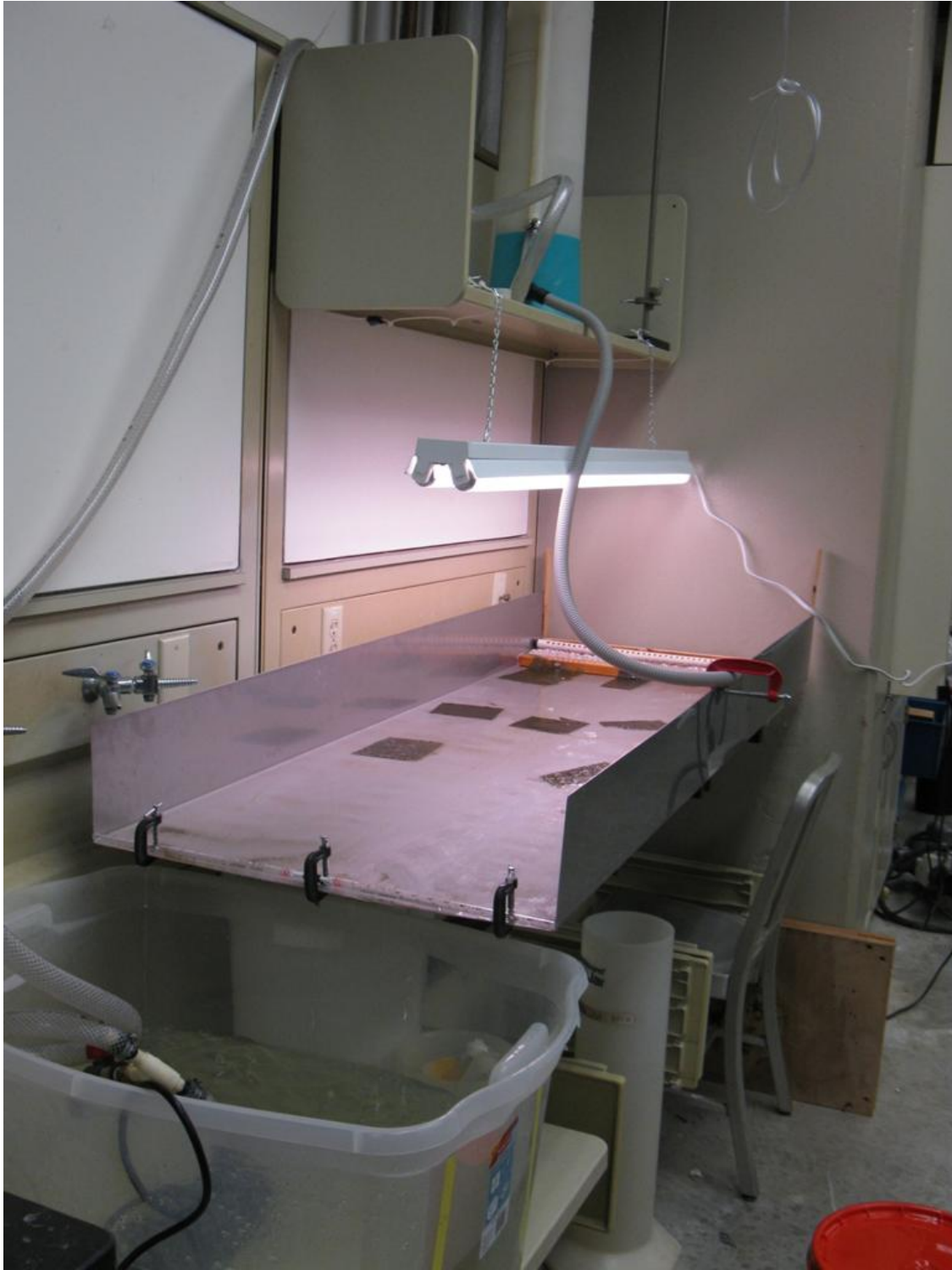
Figure 3-A.1: Photograph of bench scale algal growth flowway, seeded with sections of algae from Springdale ATS®.
