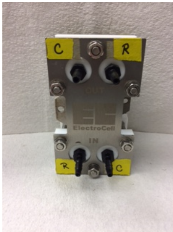
Fig. 2. Front view of ElectroCell system with 1/8" inlet and outlet connections
