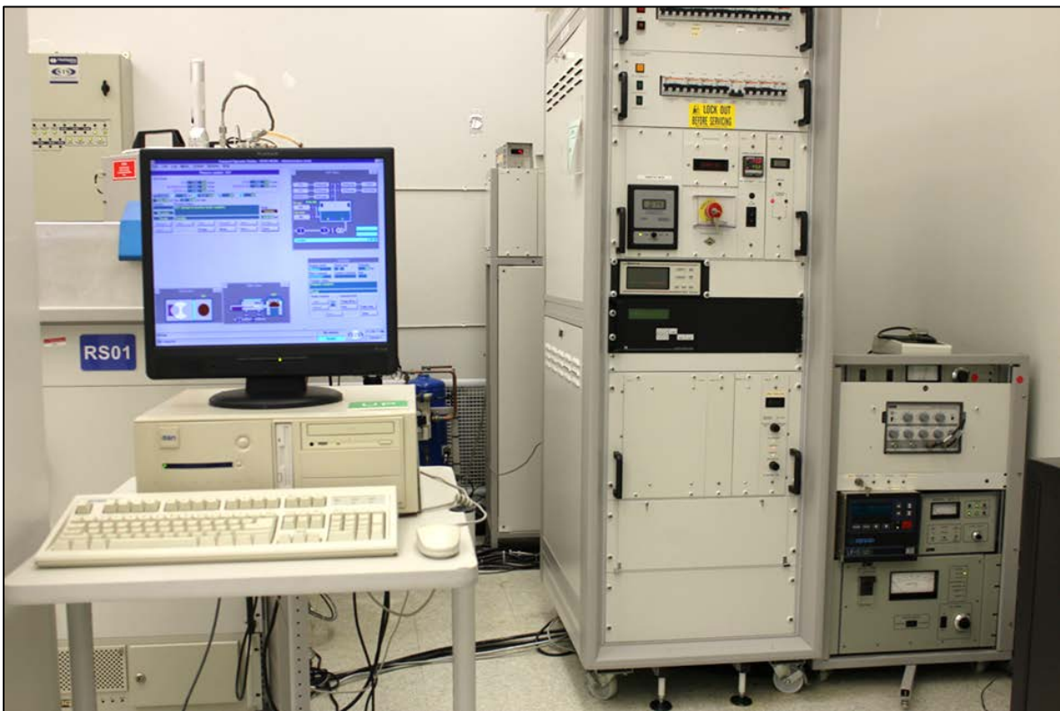
Figure 4.10. The STS ICP tool was used to etch pores in c-Si wafers ( Image from the author ).
