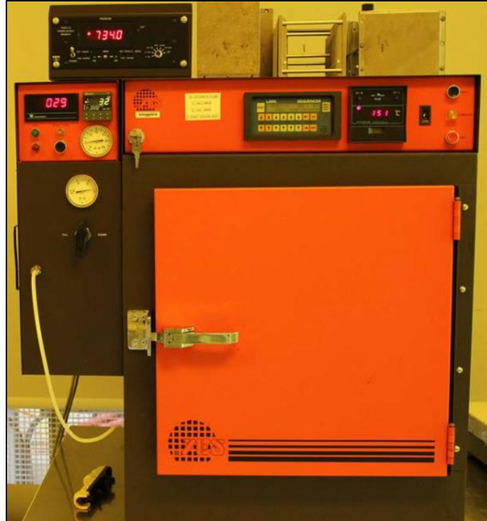
Figure 4.3. The vacuum oven was used for dehydration and application of adhesion promoter on the wafers. The room lighting was yellow to prevent premature exposure of the photoresist before photolithographic processing was done ( Image from the author ).
