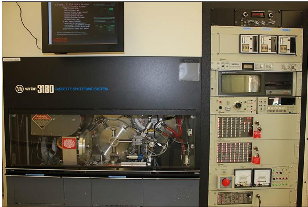
Figure 4.17. The Varian 3180 sputtering system used in the deposition of Ti, Cu, and Al films (Image from the author).
