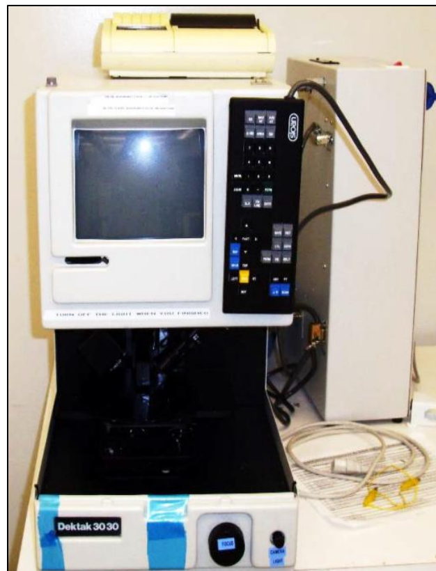
Figure 4.5. The Dektak 3030 surface profilometer was used to measure the photoresist, Cu, and a-Si:H film thicknesses throughout the photolithographic and thin film deposition processes ( Image from the author ).
