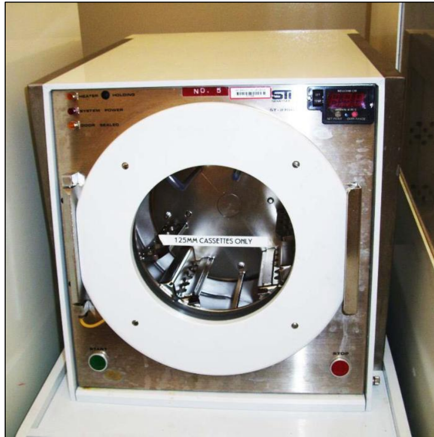
Figure 4.1. The SemiTool spin rinse and drying tool was used to remove contaminants from the surface of c-Si wafers ( Image from the author ).
