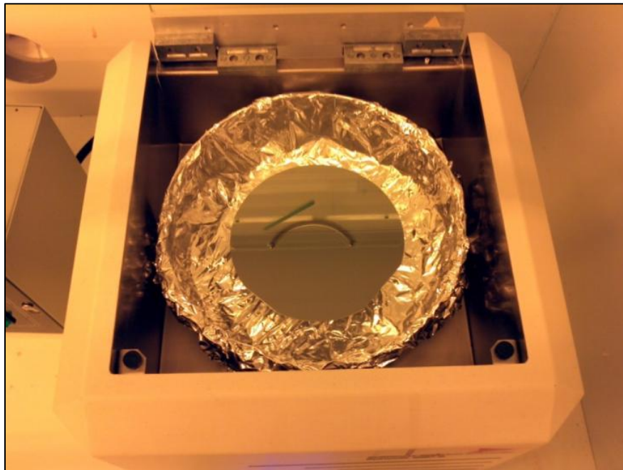
Figure 4.4. The G3P-8 spin coater was used to distribute photoresist across the wafers ( Image from the author ).
