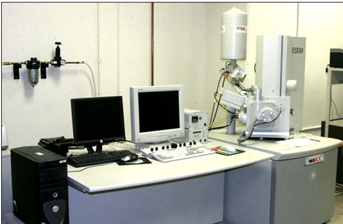
Figure 6.1. The ESEM system shown here was used to capture images of the nano-topographies [46] ( Image from the author ).
