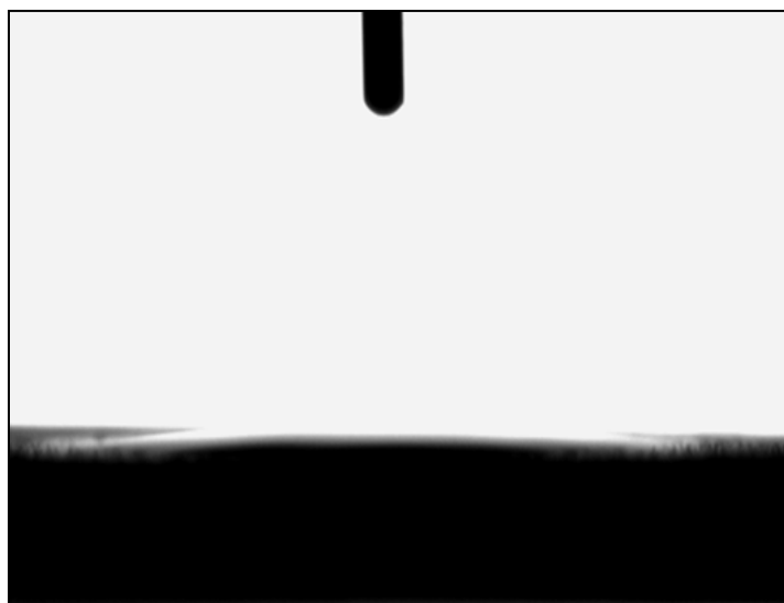
Figure 2.6. Video image of a 3 µL water droplet dispensed on the micro/nano-textured, superhydrophilic surface. The image was taken at 0.2 s after dispensing, and the WCA is about 1° ( Image by the author ).
