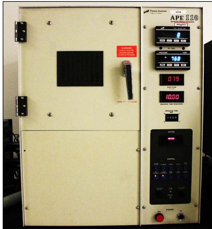
Figure 4.13. The plasma etching system was used for cleaning the wafers of photoresist remnants ( Image from the author ).
