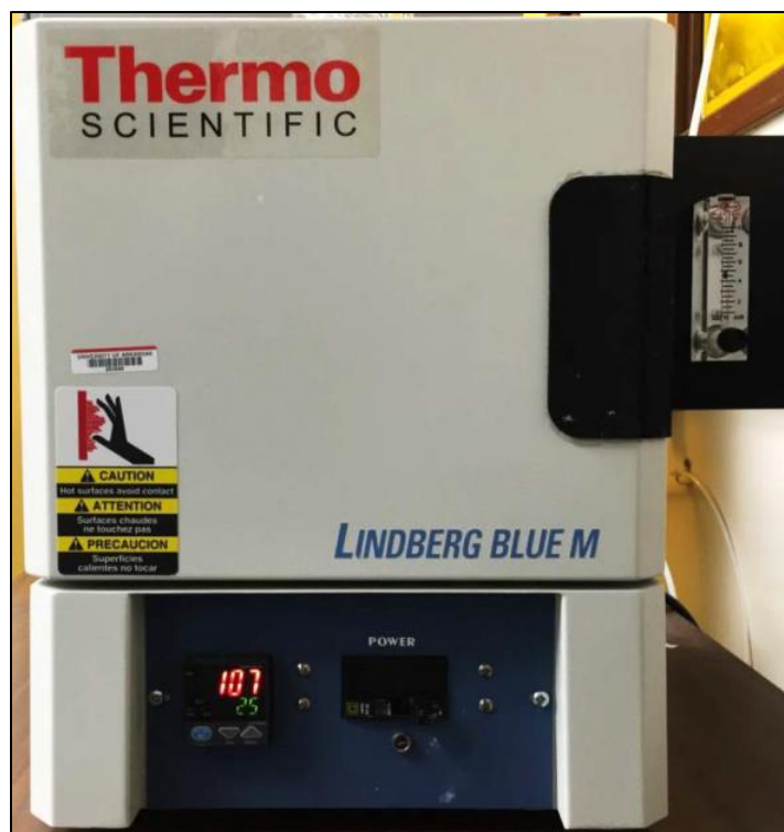
Figure 7.3. The Lindberg Blue oven was used to dehydrogenate a-Si:H film before evaporation testing ( Image from the author ).
