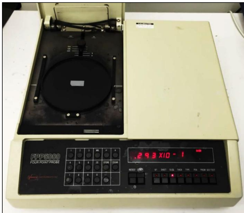
Figure 7.4. The 4-point probe instrument was used to measure sheet resistance and resistivity of hydrogenated and dehydrogenated a-Si films ( Image from the author ).
