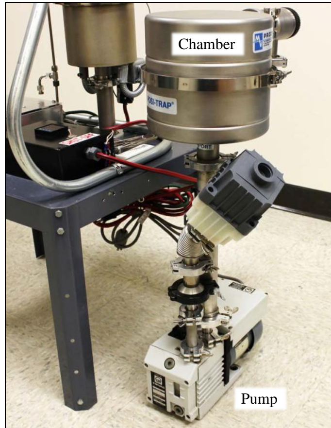
Figure 4.28. The vacuum chamber and pump used to remove trapped air from the samples ( Image from the author ).
