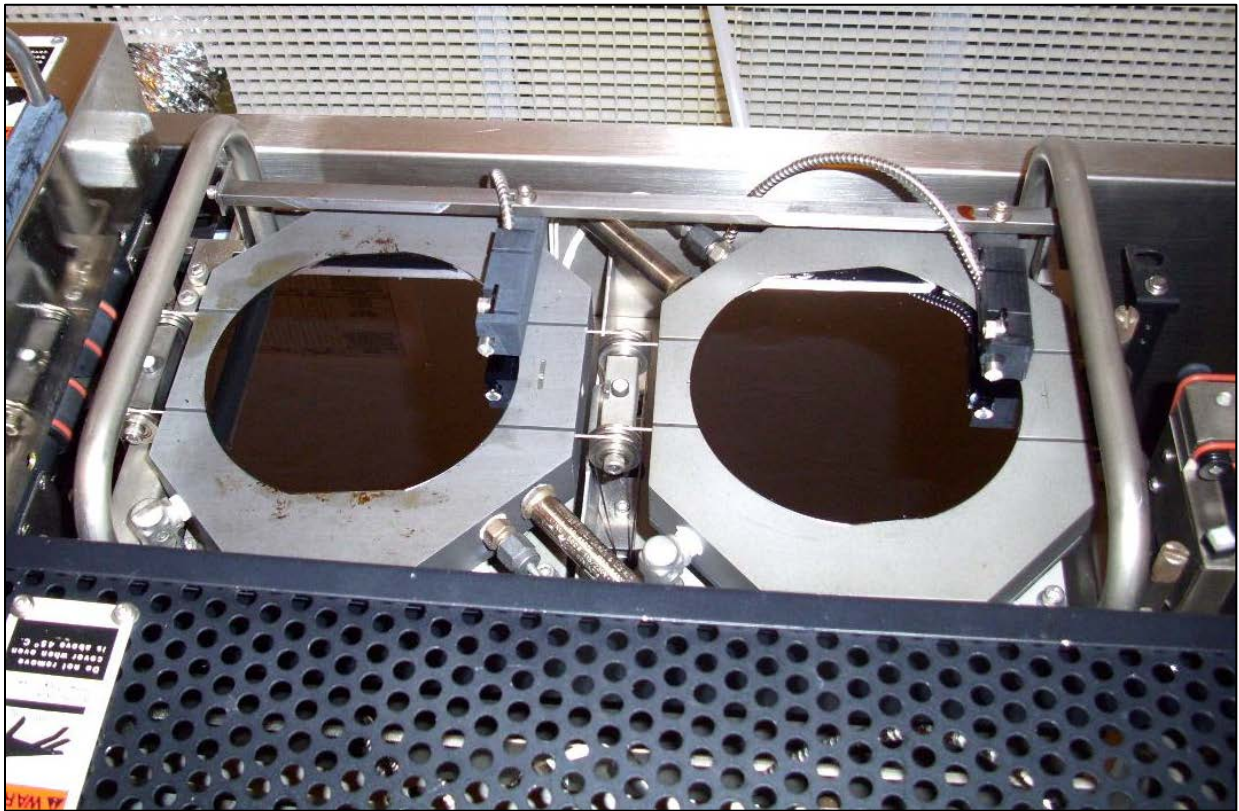
Figure 4.6. The hot (left) and cold (right) plates were used to drive solvents away, reduce stress, and promote adhesion of the photoresist ( Image from the author ).
