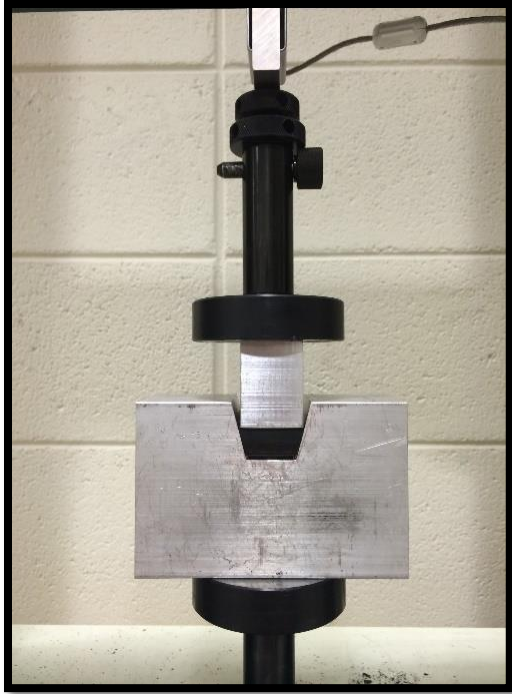
Figure 29. Experimental setup for machined aluminum block compression test.
