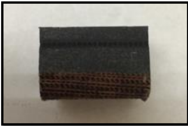
Figure 24. Prepared sample for compression test with rectangular geometry.
