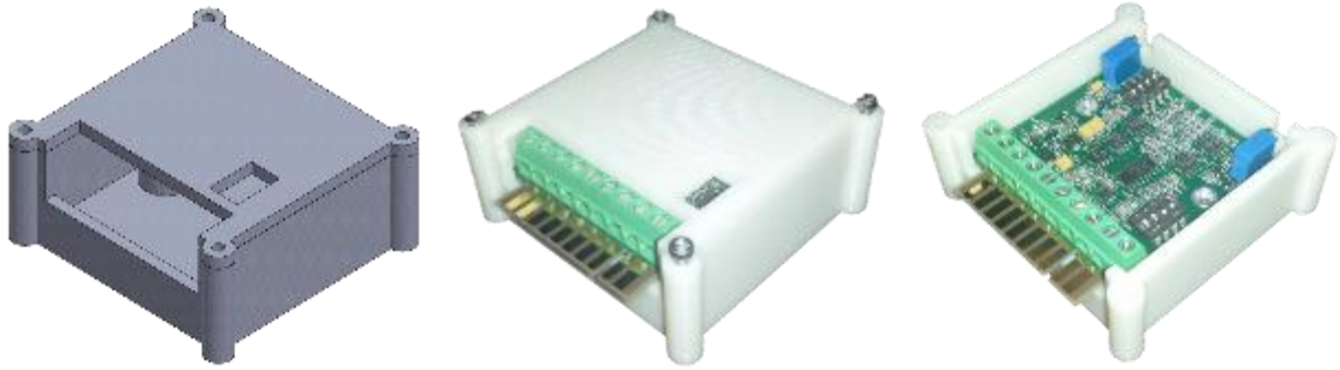
Figure 125: A 3D printed housing isolated the LVM110.
