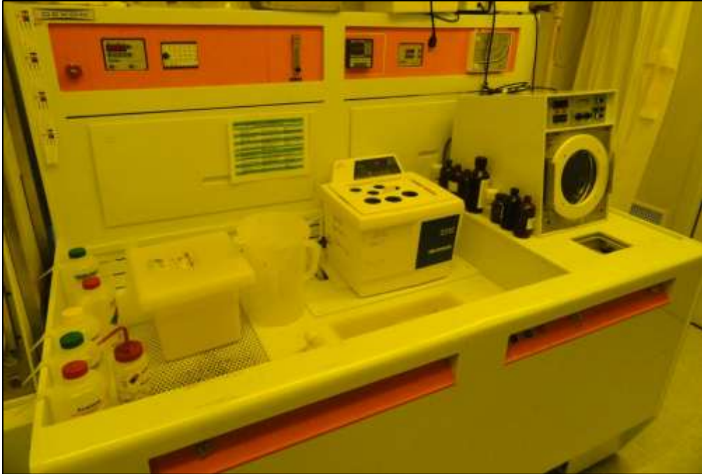
Figure 5.13: Caustic wet bench for developing PR.
