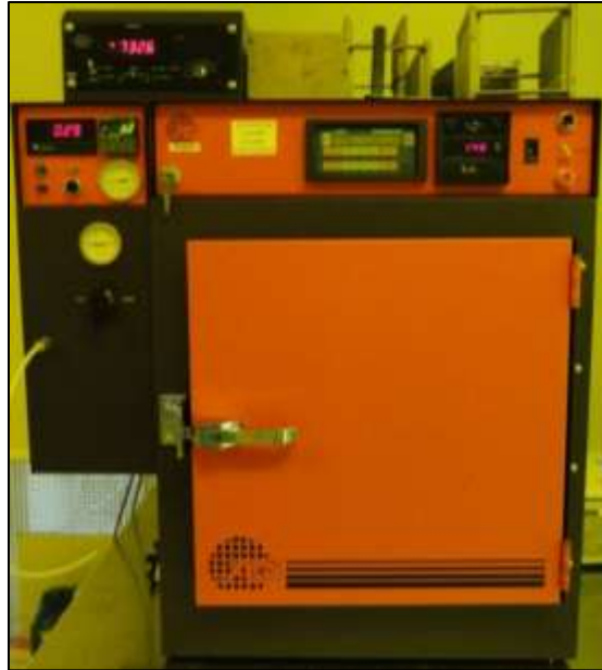
Figure 5.9: HMDS oven to generate HMDS adhesion layer in vapor form.
