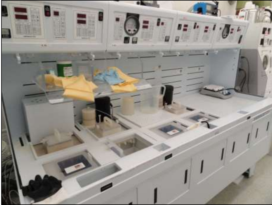
Figure 5.15: Acid wet bench for etching \text{SiO}_2 .
