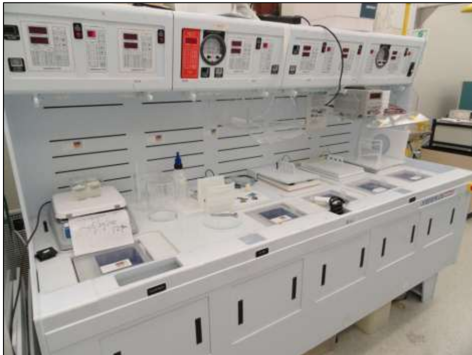
Figure 5.16: Caustic wet bench for stripping off PR.
