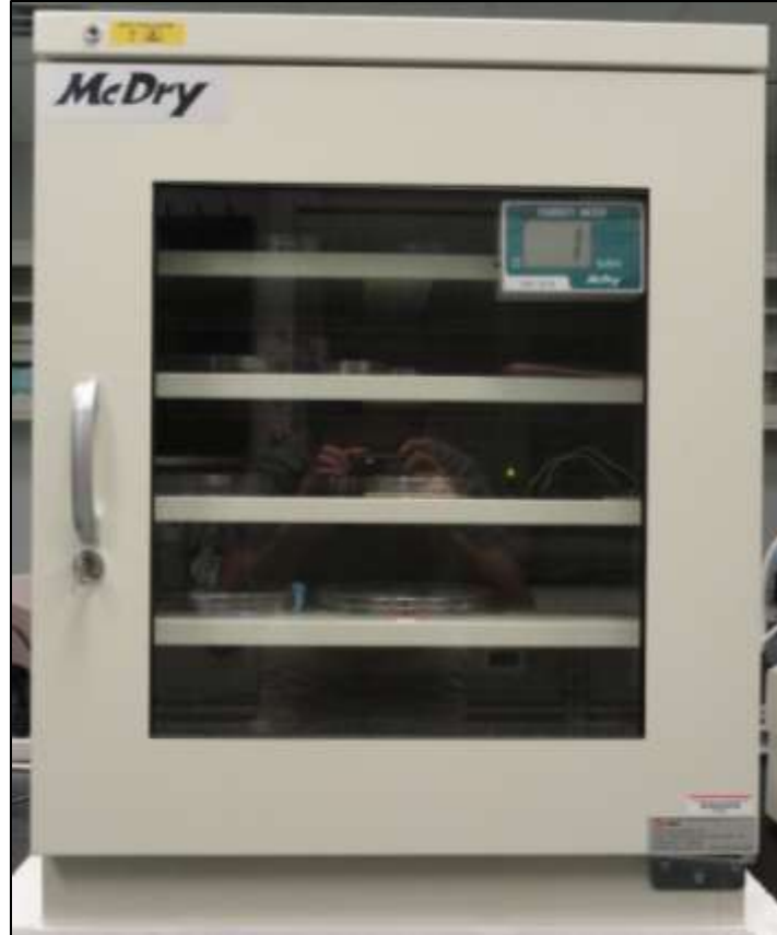
Figure 4.4: Dry box for anhydrating chip after each subzero temperature treatment.
