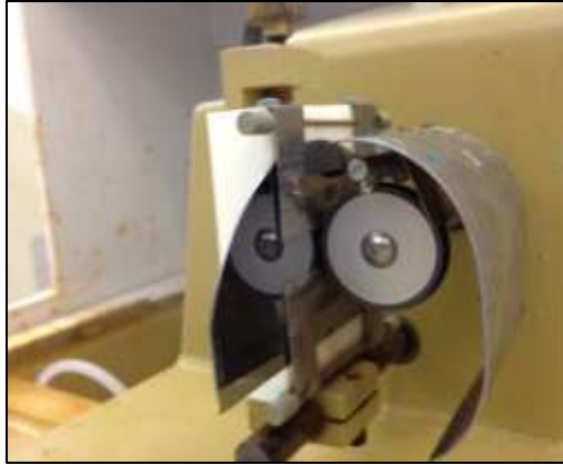
Figure 5.19: Wafer groover to fabricate groove on diffused Si substrate.
