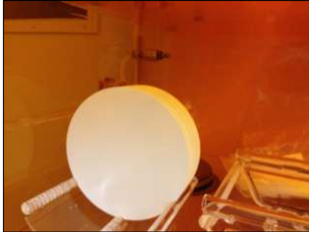
Figure 5.7: Phosphorus source wafers on boat.
