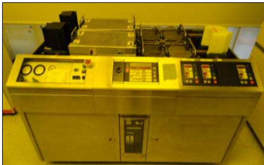
Figure 5.10: Eaton 6000HX spin coater with hotplates.
