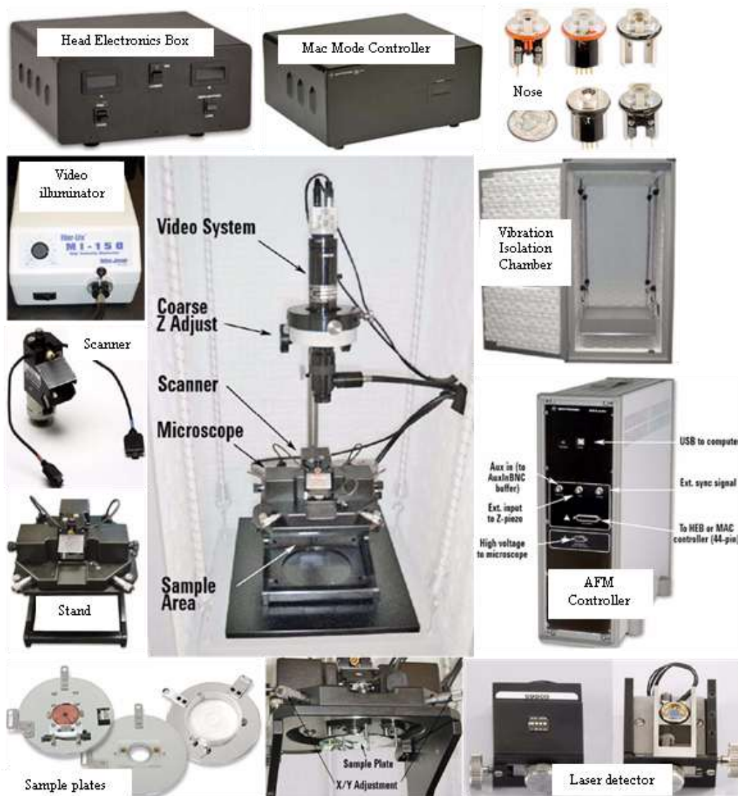
Figure 1.12: Major components of Agilent 5500 SPM.
