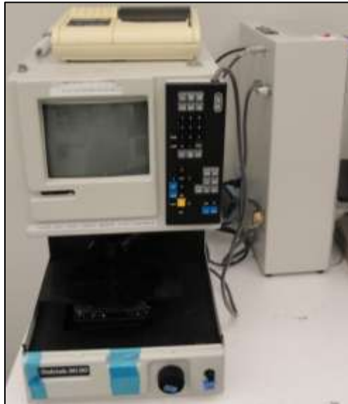
Figure 5.20: Dektak 3030 surface profiling measuring system.
