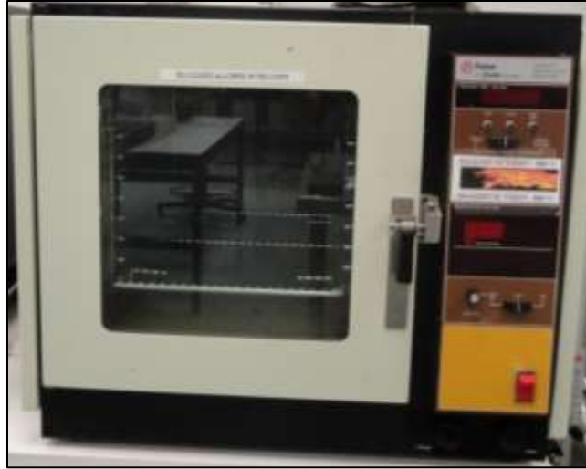
Figure 5.33: Vacuum curing oven for conductive epoxy bonding.
