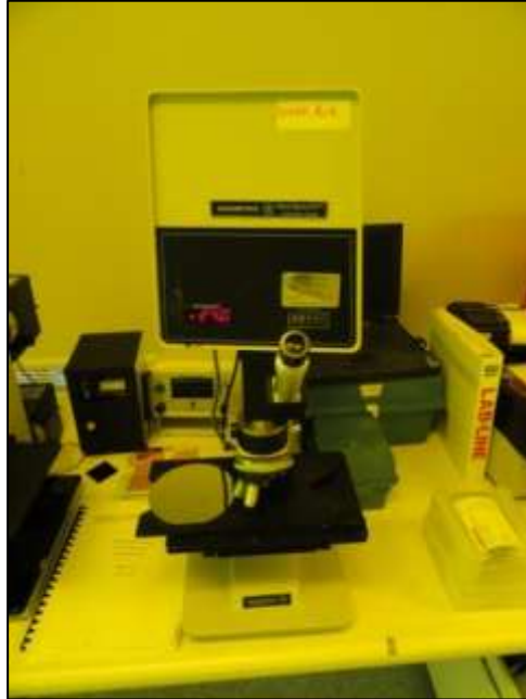
Figure 5.6: Nanospec reflectometer for SiO 2 thickness measurement.
