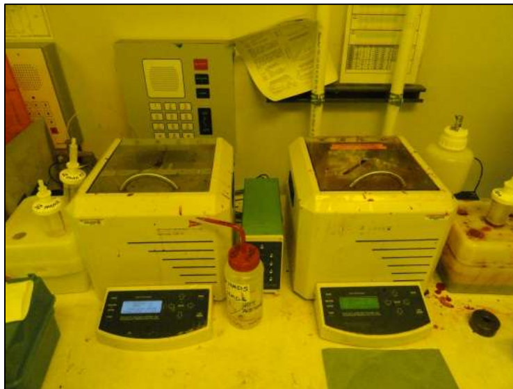
Figure 5.8: Photoresist desktop spin coaters.
