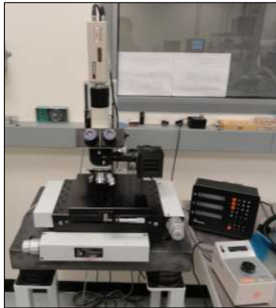
Figure 5.23: Micro measure system to measure groove dimensions.
