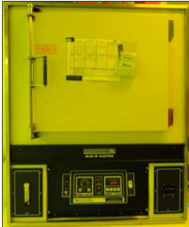
Figure 5.14: Blue M Oven for baking PR applied to wafer backside.
