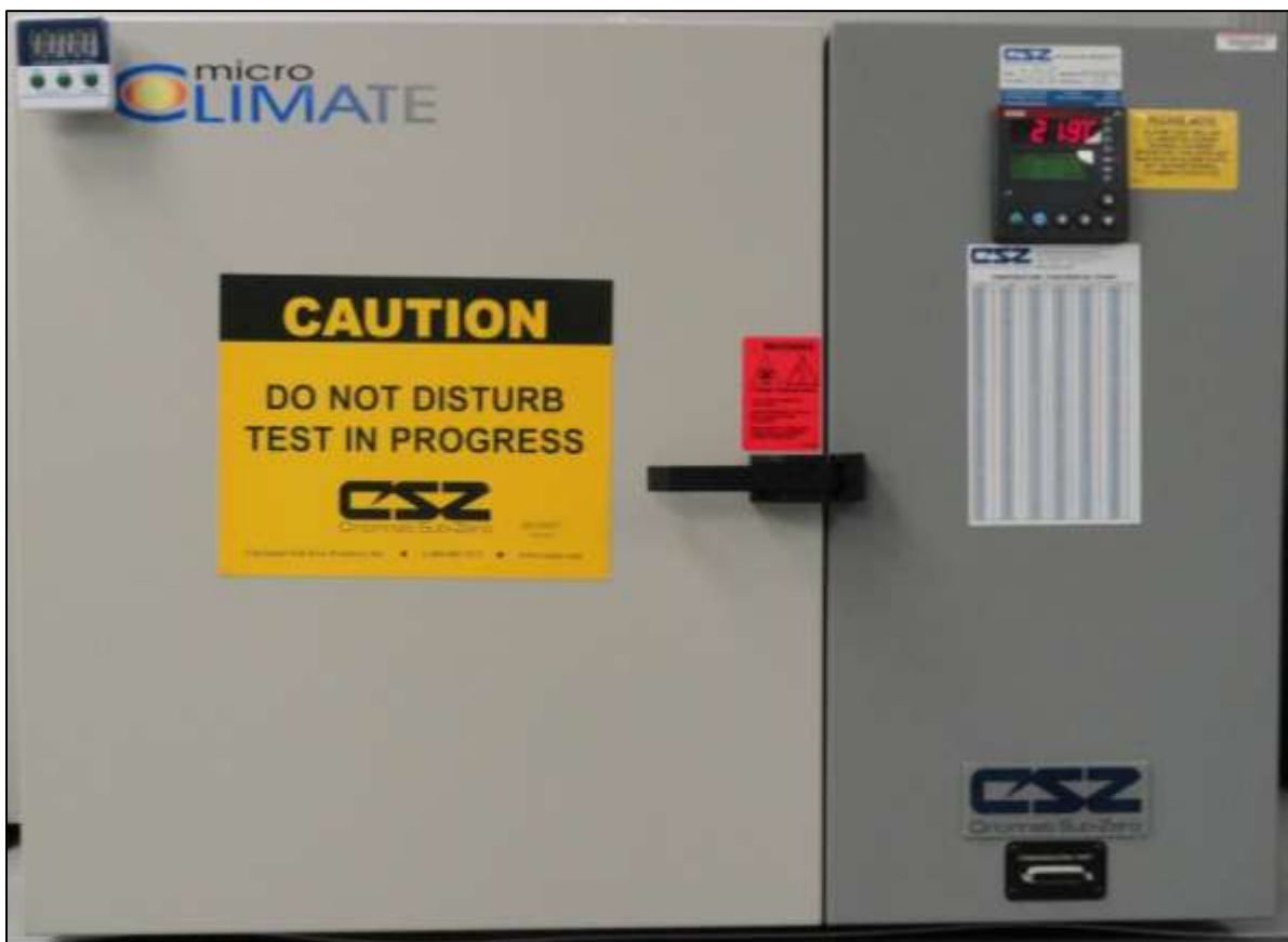
Figure 4.3: Microclimate benchtop test chamber for subzero temperature treatment.
