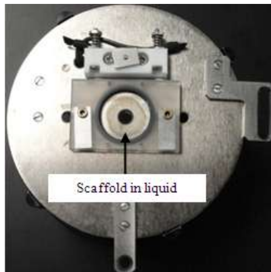
Figure 4.11: Liquid cell for imaging and indenting samples in liquid.
