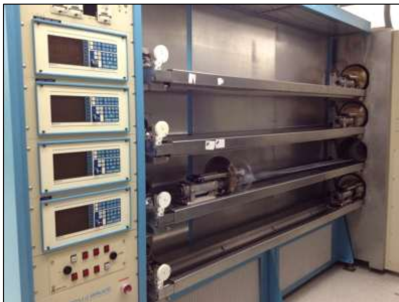
Figure 5.5: Diffusion furnace for oxidation and diffusion.
