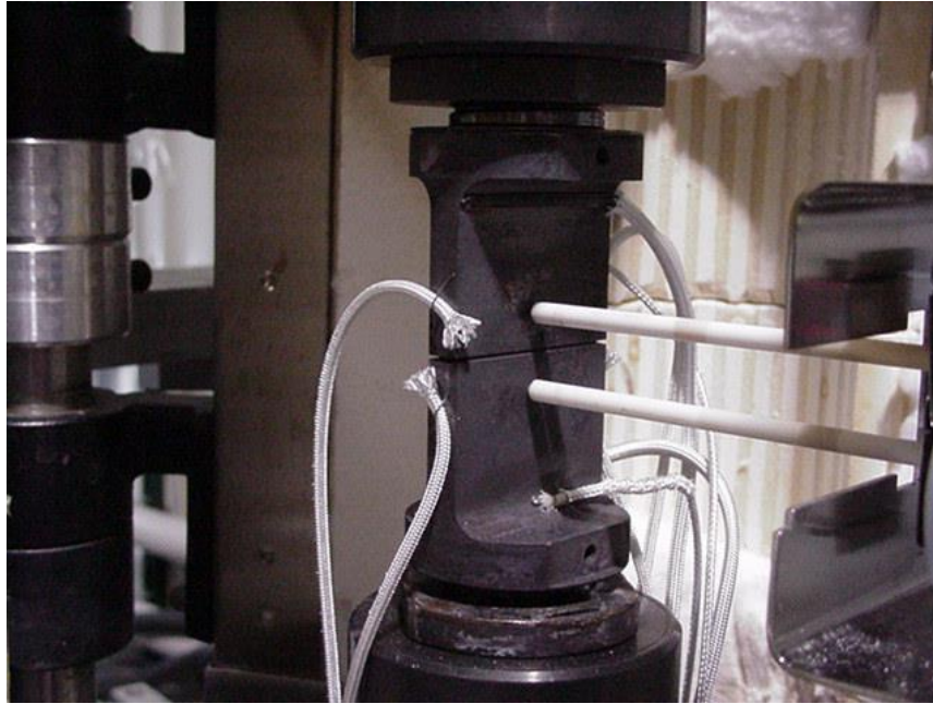
Figure 10.1. HT extensometer mounted directly on the load-line of DEN(T-C) specimen. Courtesy of WMTR, Youngstown, PA.
