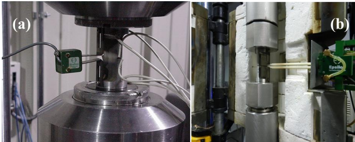
Figure 8.2. Schematic of measuring load-line deflections in DEN(T-C) specimens.
