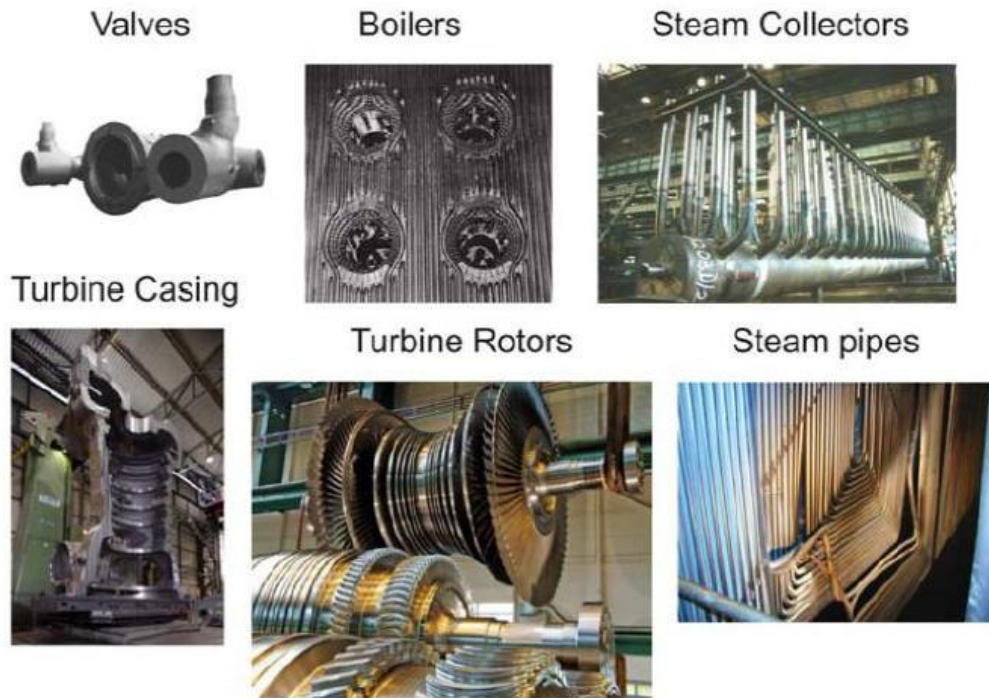
Figure 5.1. Various applications of the 9-12% chromium martensitic/ferritic steels in the fossil-fired steam power plant industry [80].
