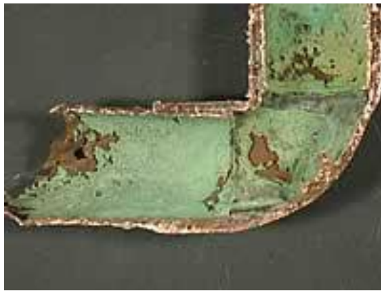
Figure 9 Erosion-corrosion inside of copper alloy pipe (Courtesy Midland Corrosion Associates)
