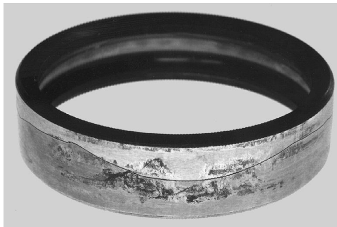
Figure 10 Fretting corrosion on the outer ring of bearing (Courtesy Maintenancebits, SKF group)
