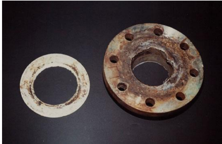
Figure 5 Crevice corrosion (beneath a seal) on a stainless steel flange exposed to a chloride-rich medium (Courtesy Multimedia Corrosion Guide)
