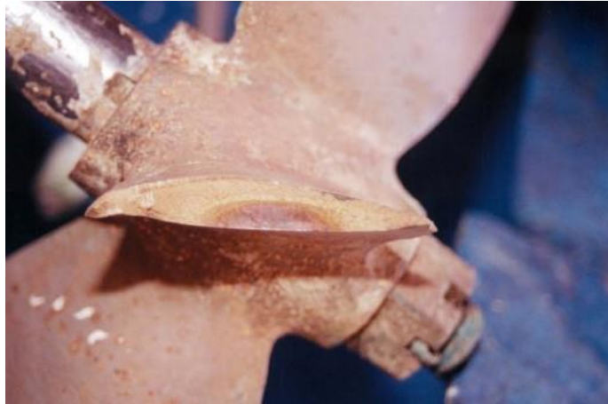
Figure 8 Dezincification of brass propeller blade (Courtesy Jim Aleszaka, Fracture Investigations Inc.)
