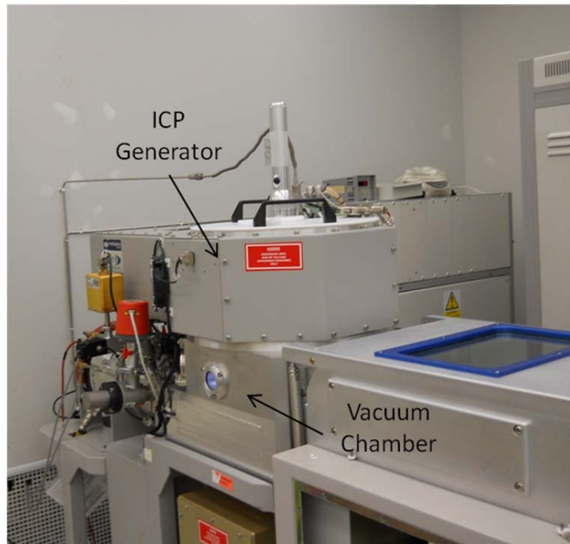
Figure 6: The DRIE used for low SFE fluorocarbon film deposition.
