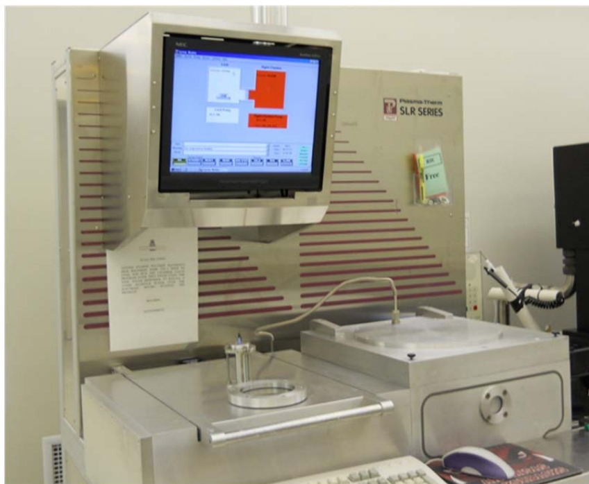
Figure 4: The PlasmaTherm SLR RIE used for oxygen plasma treatments.
