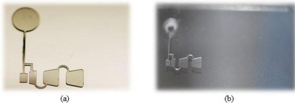
Figure 3.7 (a) SU-8 mold on Si wafer for thin PDMS control layer (b) A thin PDMS control layer
