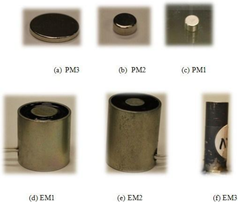
Figure 4.18 (a) to (c) Permanent magnets (d) to (f) Electromagnets for magnetic separation of SCP beads
