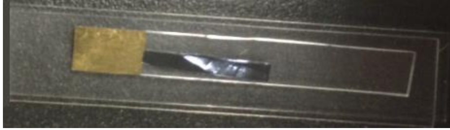
Figure 62-Testing Setup of Thermal Tape to be Heated on the Sensing Substrate
