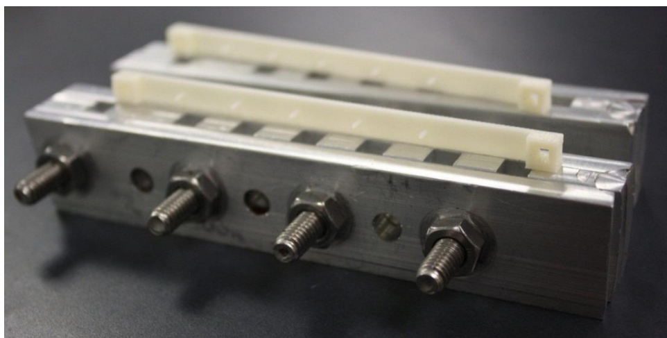
Figure 14: Mold used for fabricating all of the samples used in this thesis work
