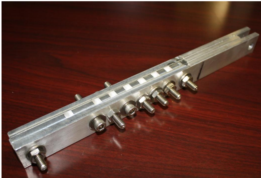
Figure 13: First iteration of the aluminum mold for the PDMS test sample
