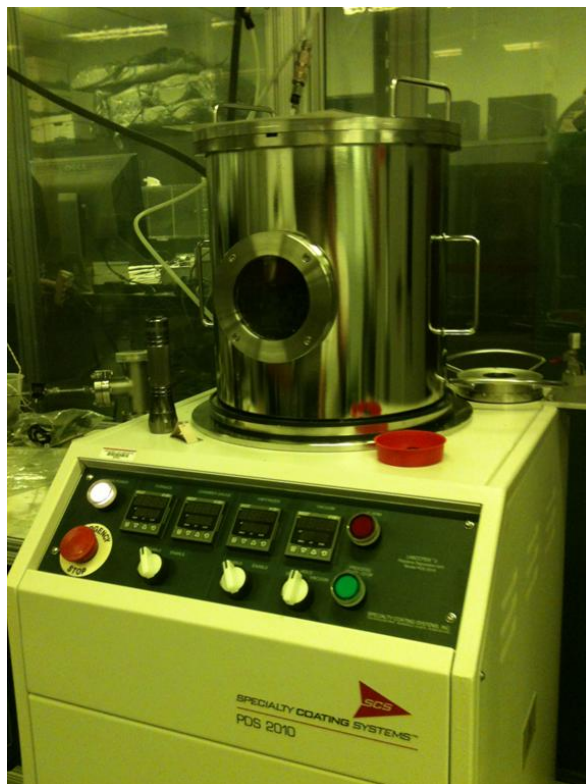
Figure 16: Parylen coater camber model PDS 2010 manufactured by Specialty Coating System used to degas the samples.
