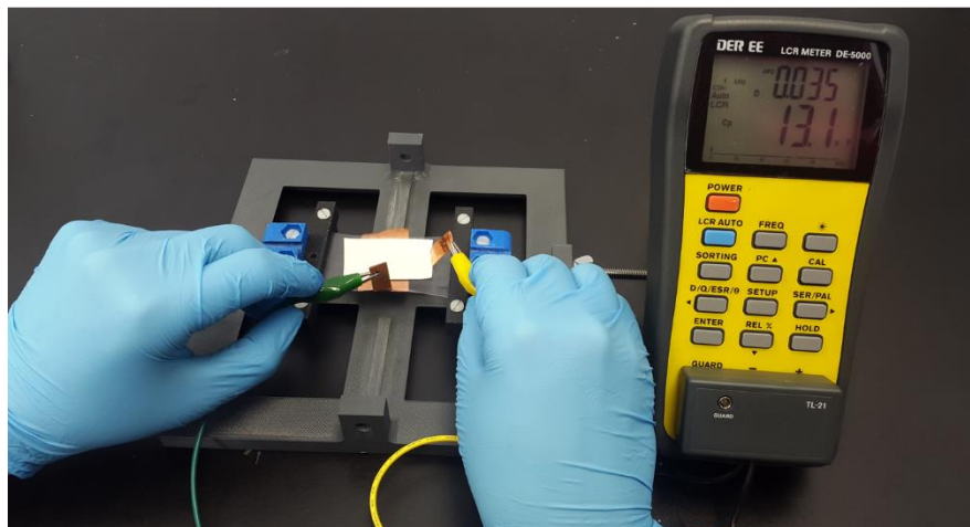
Figure 23. Dielectric constant measurement for printed silicone elastomers
