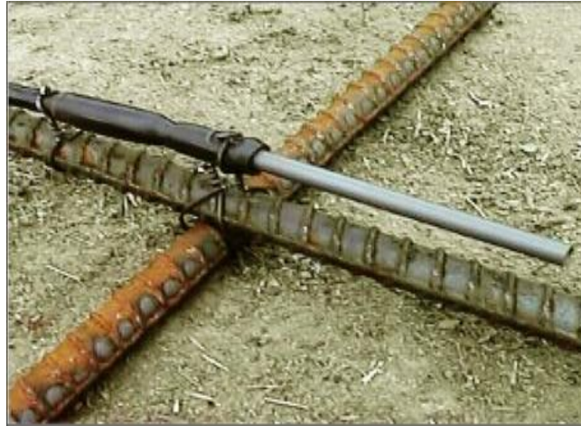
Figure 2: Example of a probe installed inline on the sample to monitor. [3]
