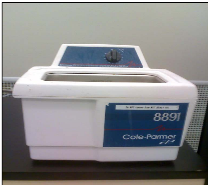
Figure 3.2. Ultrasonic cleaning apparatus used in the preparation of samples for nano-texturing [49].
