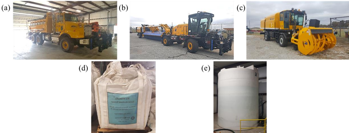
Figure 69: XNA snow removal equipment and pavement treatment chemical; (a) plow truck/chemical spreader, (b) multi-tasking vehicle, (c) snow blower, (d) sodium formate/acetate pellet deicer, (e) potassium acetate/propylene glycol liquid deicer.
