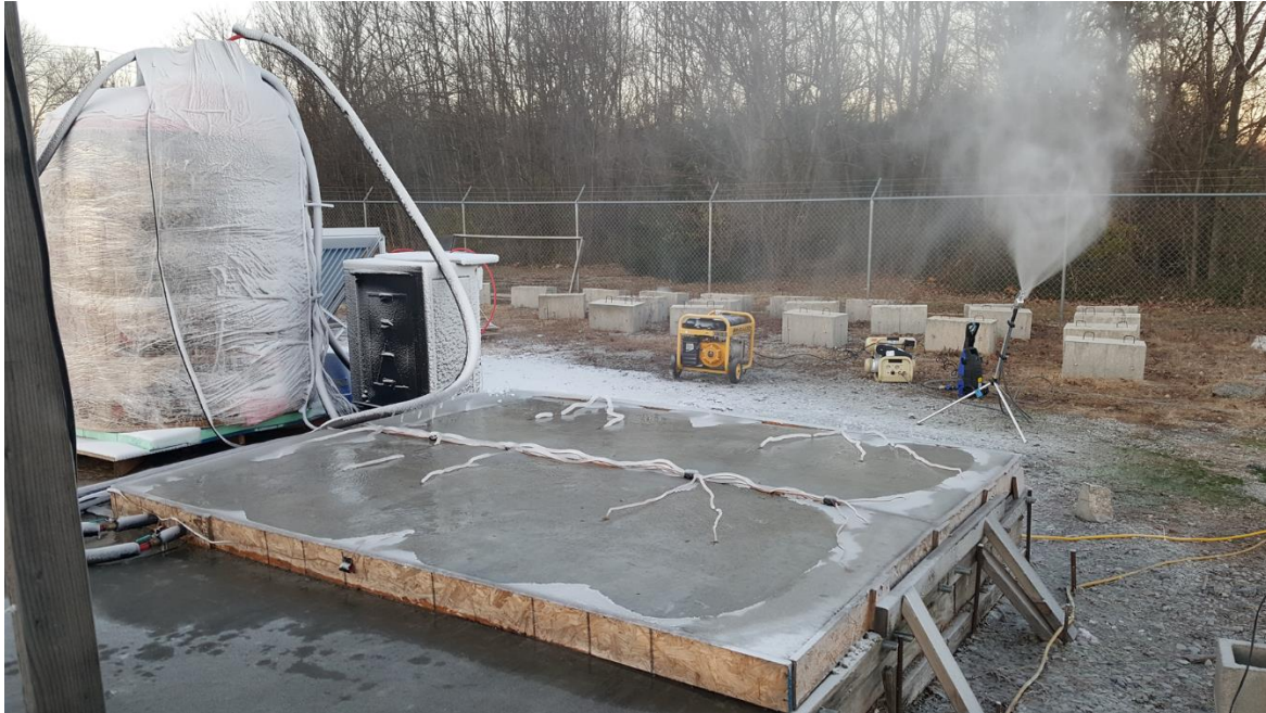
Figure 111: Snowmaking machine positioning for anti-icing tests.
