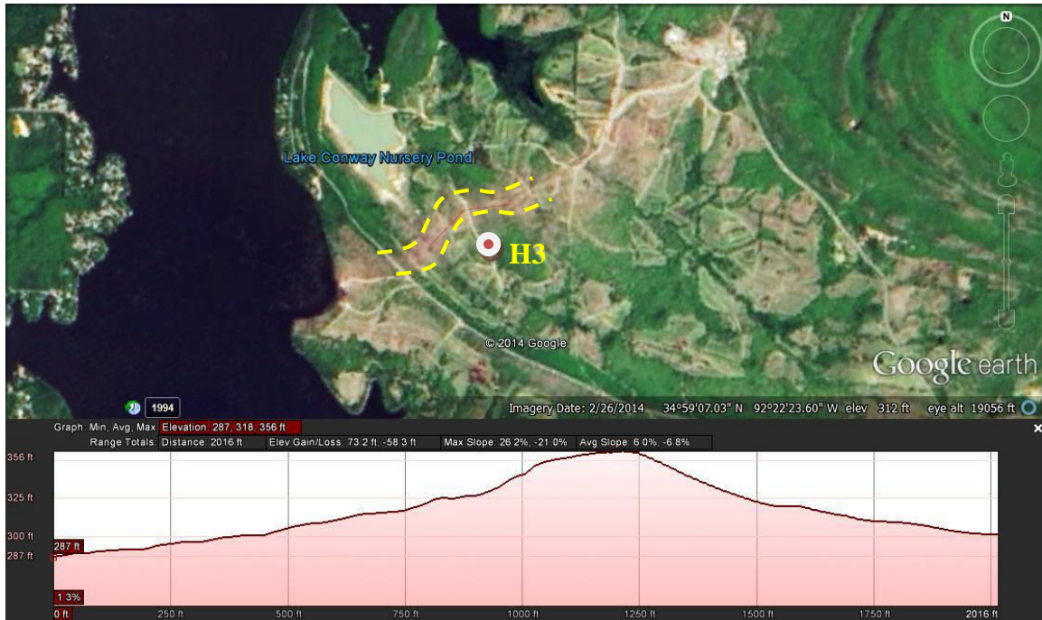
Figure 6.11 Elevation profile for the hill in location H3, ( V_{\theta}/V_t \approx 4 , single curvature).
