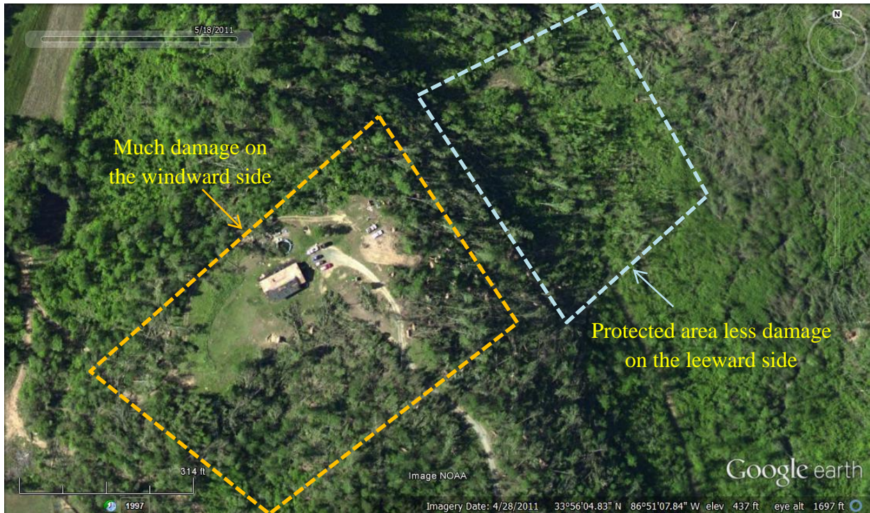
Figure 4.8 Close-up view for hill (H4), much damage on wind ward (the faded brown area, yellow line) and the protected area on the leeward (dark green, blue line).
