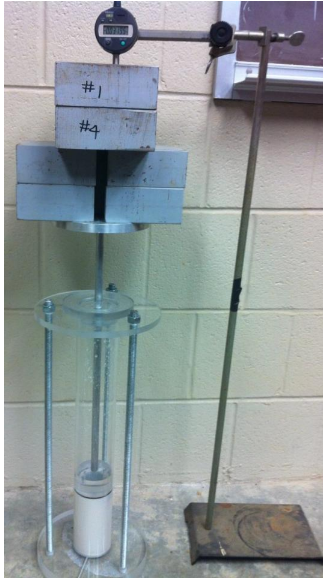
Figure A.15. Laboratory prepared Kaolinite sample from a slurry consolidometer at the University of Arkansas.
